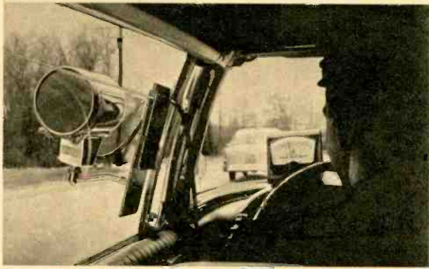
In-car components of Doppler speed-trap system are surprisingly few. Gauge directly in front of officer shows speed of car ahead.
