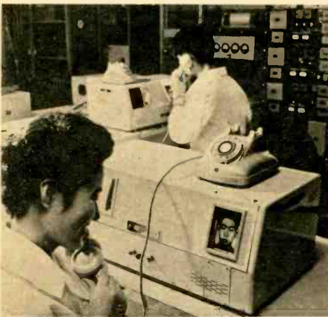
Talk/see device developed by Japan's Tokyo Shibaura Electric can be attached to any telephone, sends a still picture over existing telephone lines.
