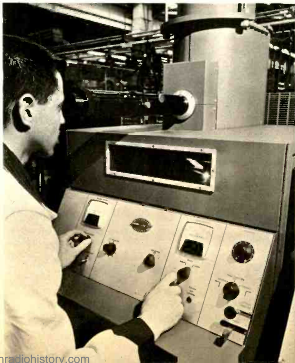
Electron-beam welder has telescope-type viewer so operator can see what's happening to workpiece.
