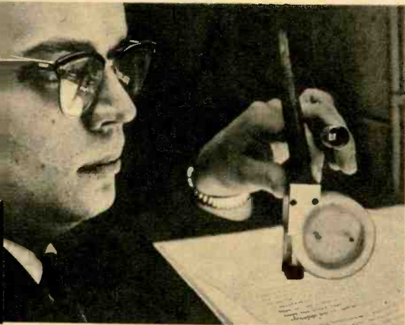
Fiberscope will transmit image from end to end whether it's curled in a loop or lying straight. See letters in viewer between the man's fingers.
