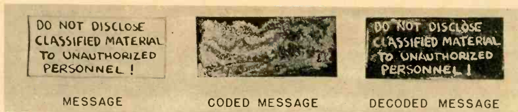
Message becomes hash in scrambled optical fibers, can be decoded only by special decoding fibers.
