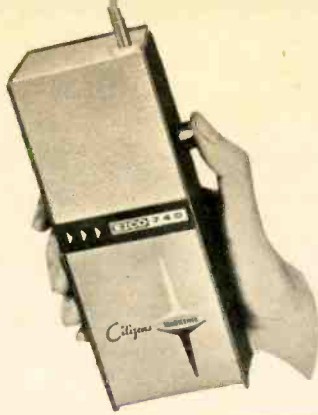
EICO Model 740 handi-talkie offers 100-mw transmit power, has 1 crystal receive channel. Nine transistors; kit. $54.95.
