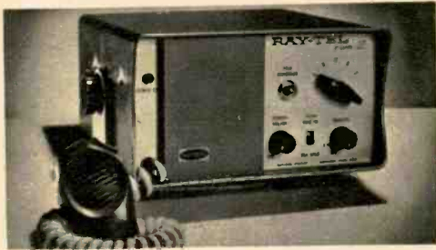
Ray-Tel 2 is a business rig offering 5 channels without variable tuning. It has adjustable squelch, noise limiting, 10 tubes, 117-VAC or 6/12-VDC operation. Comes with a yoke mount. $189.95. Raytheon Co., Lexington 73, Mass.
