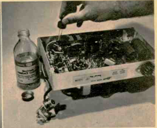
Transmit and receive switches require periodic cleaning for trouble-free operation. A liquid cleaner is being used here; never file contacts.
