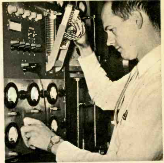
CREI GRAD ROY A. REICHERT makes an adjustment on the prototype of a programmable power supply which he designed and built in his capacity as Senior Technical Aide, Bell Telephone Labs, Murray Hill, N. J.
