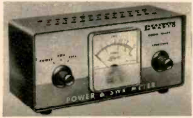
Lafayette TM-58 is an SWR bridge and RF power meter which can be inserted permanently in the coax line. It indicates up to 15 watts power, has a built-in dummy load, measures SWR from 1:1 to 4:1. $7.95. Lafayette Radio, Syosset, N. Y.
