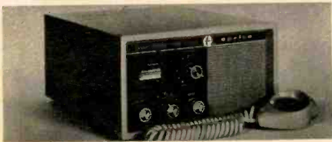
Apelco AR-10 is a 10-channel job with noise limiter, squelch, and combination modulation-output meter. It has 3 IF stages, operates on 117 VAC or 12 VDC. Meets DOT specs for use in Canada, maker claims. Apelco, S. San Francisco, Calif.
