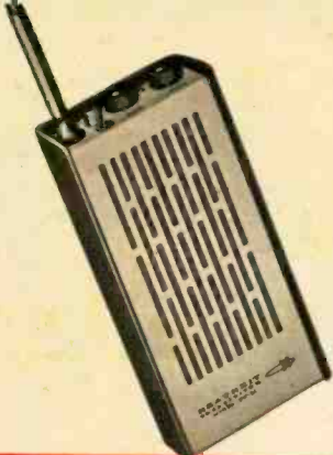
Heath GW-21 is a 9-transistor handi-talkie. It has 1-channel superhet receiver. Transmitter is rated at 100 mw. Kit, $44.95.
