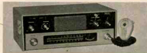
Heath GW-42 is a kit which includes 3 circuit boards. It has a 3-way power supply, 5 crystal T-R channels, four-tone selective call, slide-rule dial, meter, noise limiter, squelch. Price is $119.95. Heath Co., Benton Harbor, Mich.
