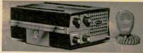
Pearce-Simpson Companion features 5 crystal T-R channels, noise limiter, squelch, 3 watts actual RF output. Modulation limited to 95%. Cabinet is 8 3/4 x 12 1/4 x 5 inches. Price is $189.50. Pearce-Simpson, Miami 35, Fla.
