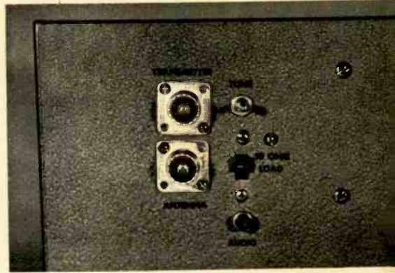
Side panel rear showing jacks J1, J2, load switch S2 and input coil L1's slug tuning adjustment.
