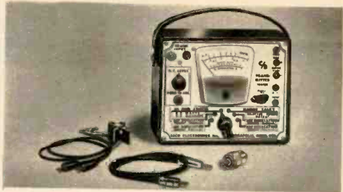
Seco 510 Transmitter Tester is a portable instrument which gives you a direct reading of percentage of amplitude modulation and actual RF output. High impedance input for handi-talkie checks. $46.95. Seco, Minneapolis 19, Minn.
