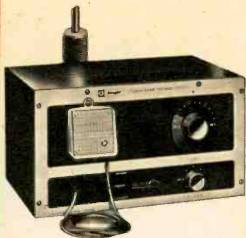
Allied's Knight-Kit C-11 rig features tunable superregen receiver; 1-channel, 5-watt transmitter. Kit price is $39.95.
