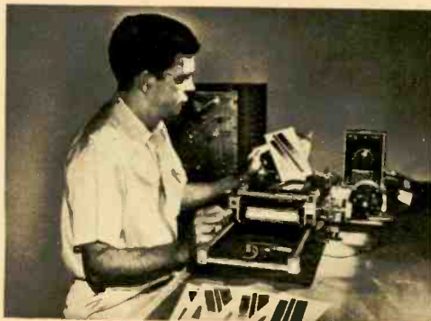
Prototype of the electronic printing machine. Note the DC power supplies in rear of picture.
