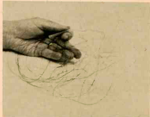
A HANDFUL— A complete 50-foot antenna with one insulator; the antenna runs directly to the rig.
