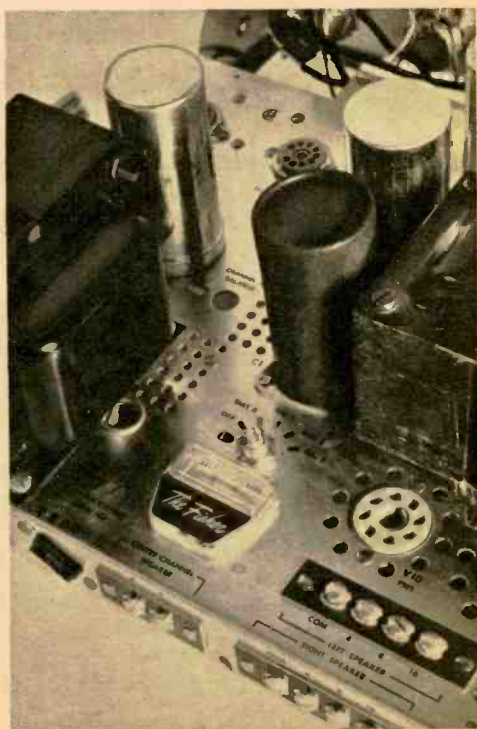
Close-up of chassis rear shows metering provisions and center channel speaker output. Five-position switch immediately above meter selects its function (either bias or balance) for each channel.
