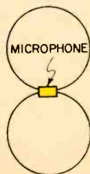
Fig. 2—Polar diagram of the bi-directional microphone's pickup.
