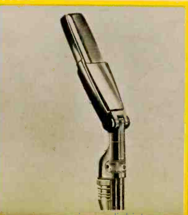
The Shure 300 ribbon microphone has flat frequency response from 40-15,000 cps, is bi-directional.
