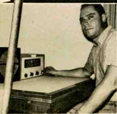
Author tuning 152-174 mc rig; note simplicity of equipment. Antenna above is 36 in. long.
