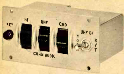
Capsule's tiny audio control panel has vertical thumbwheels, Morse code button, function switch.
