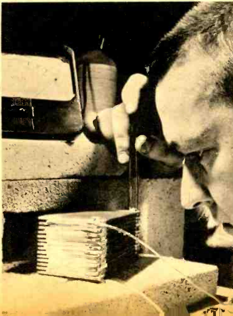
All-ceramic thermoelectric generator turns out 100 volts when heated in oven to 2,400 degrees.
