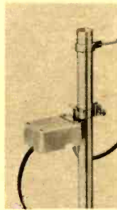
Antenna amplifiers soup up a signal before it enters downward. A good one costs $30 to $40. Models shown are by (top to bottom) Winegard, Channel Master, Jerrold and Blonder-Tongue Labs.
