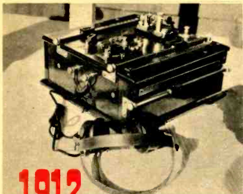
United Wireless Telegraph "D" receiver of 50 years ago had three tuning coils with sliders, used a crystal detector. Cabinet was of mahogany.
