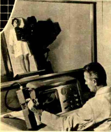
Wedding of remote-control fluoroscope and closed-circuit TV gives a doctor X-ray eyes to see such things as this young lady's stomach.
