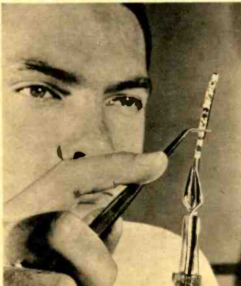
Radiation detector on tip of instrument stick goes right into patient's vein for isotope measurement.
