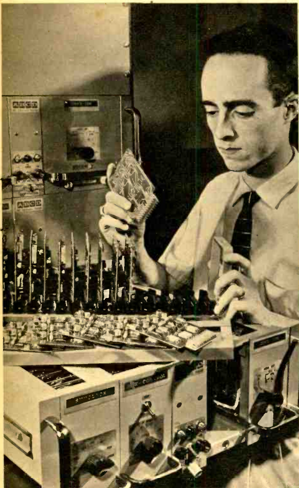
A building-block approach is taken by ACF Electronics in putting together data transmission equipment. More modules, such as the one held by the engineer, mean more complex computers.
