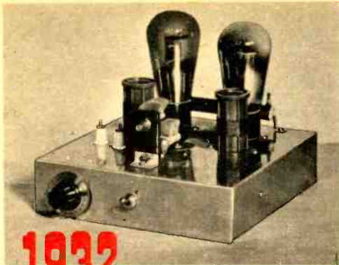
Popular early-Thirties transmitter had triode oscillator working into triode amplifier; note "new" metal chassis just then coming into general use.
