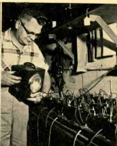
2 . . . Clustered motors are run in on bench to assure stable operation. A Strobotac is used periodically to check on rpm of individual motors in group.
