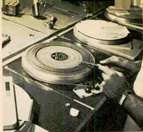
5 . . . Just before cover is put on the assembled turntable it gets a stroboscope speed test to make sure it operates in certain narrow limits.
