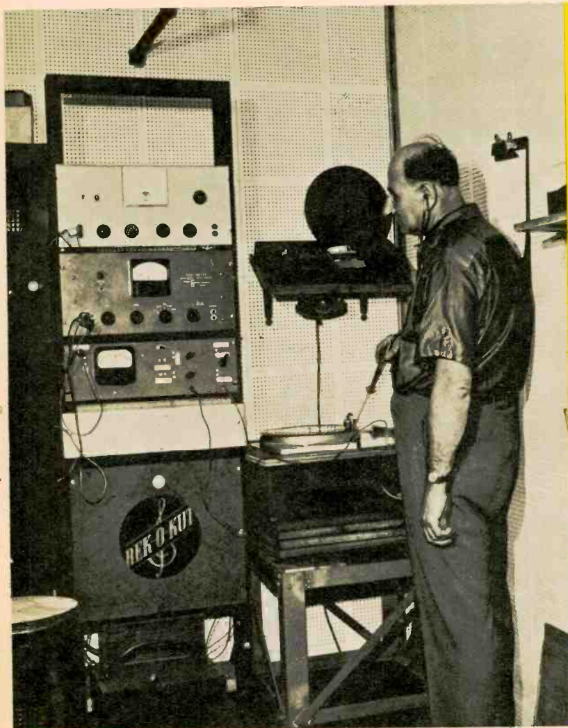
6 . . . In the last step before it is shipped out, new-born turntable plays while a worker uses stethoscope to listen for rumble and other possible ills. The panel instruments check wow, flutter in assembly.
