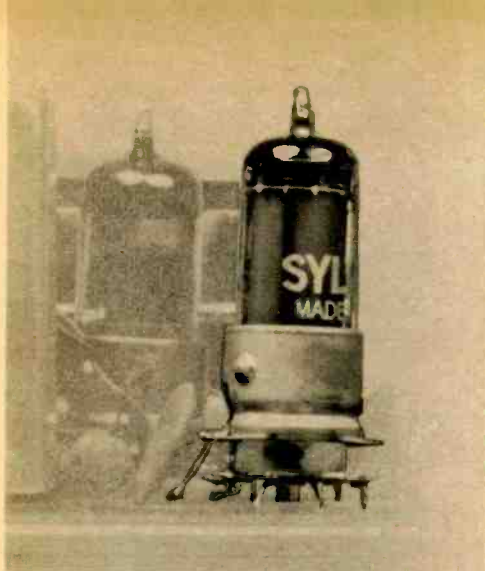
Closeup of tube socket mounting. Note bent lugs and bare wire soldered to metal socket shield.
