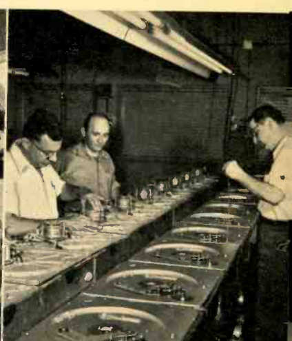
3 . . . Skilled workers on the assembly line put together the components to make up two types of hi-fi turntables. Supervisor is in background.
