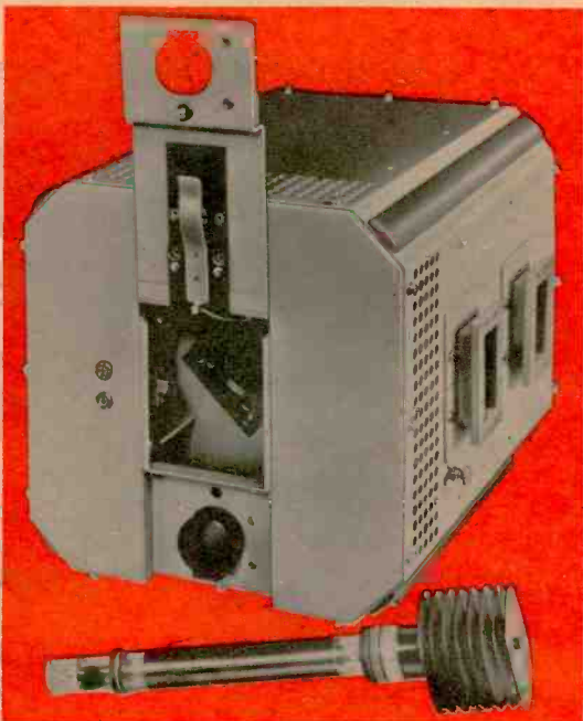
A traveling wave tube by Amperex lies in front of its complicated socket, or mount. It is an amplifier in 3800-4200 mc range.
