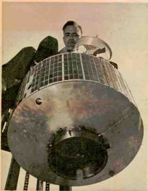
Solar cells, 2700 of them, surround satellite. They power communications repeater system.
