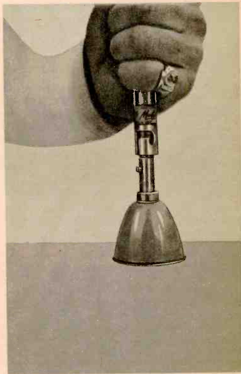
Spring-loaded Quick-On Connector accessory allows the whip to be disconnected from the base when boat approaches a low obstruction.
