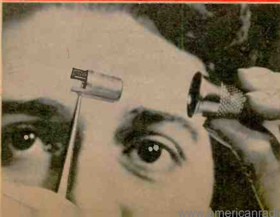
Smallest electron tube is the Nuvisor, which fits neatly into thimble. It has ceramic-metal construction and can take big temperature changes.
