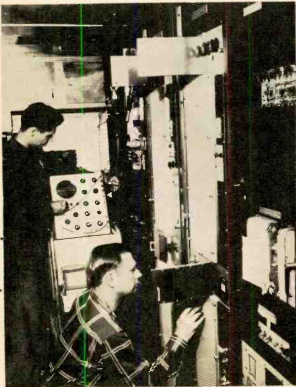
Incoming meteor burst signal of high-speed data shows on oscilloscope, left, is recorded on tape at right, fed at low speed to teletype.
