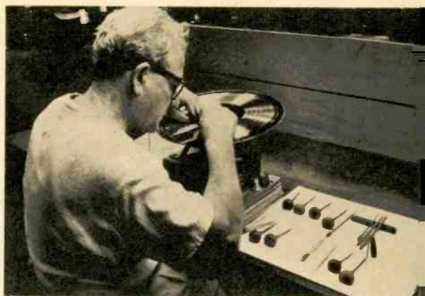
7. Mother is retouched if blemishes appear. Stampers are made from mother in next step.
