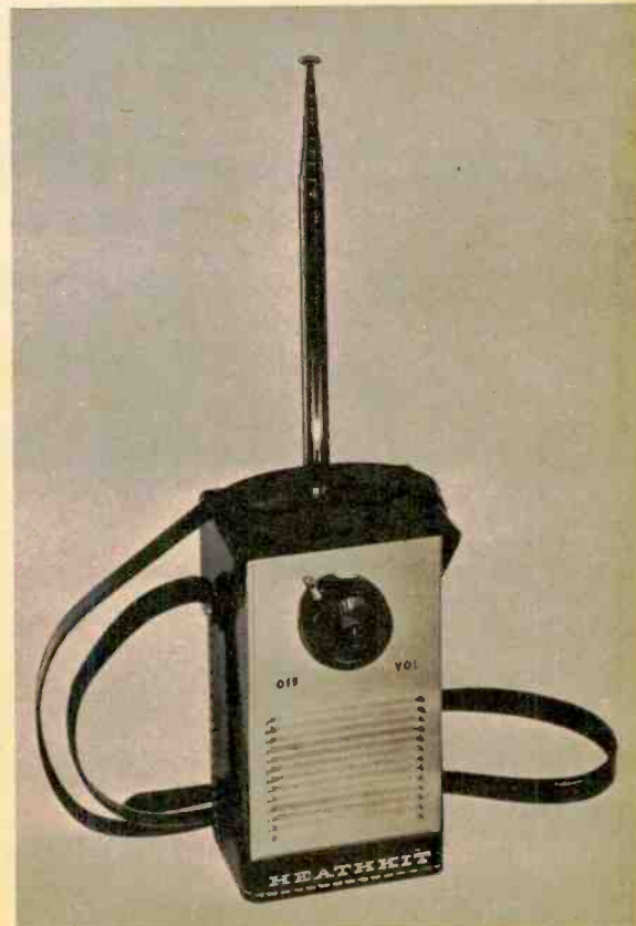
Transceiver carrying case. Whip antenna may be collapsed or removed from the unit.
