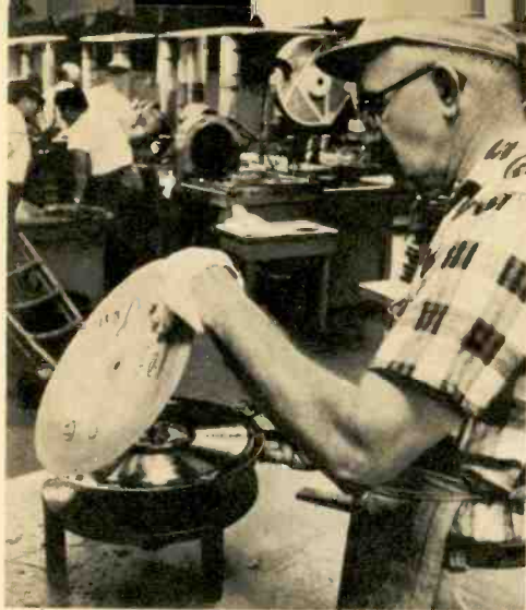
6. Copper negative is stripped off. Positive copper "mother" is made next from the master.
