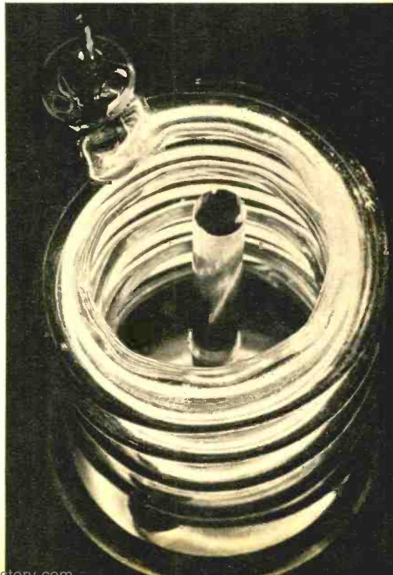
"The works" of a light maser. Light radiates from one end, is absorbed by shield at the other. Ruby ends are polished optically flat.
