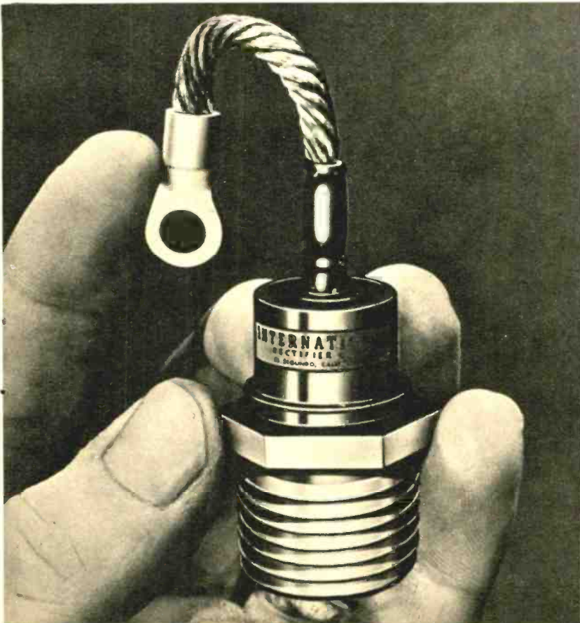
A high power silicon rectifier with current rating in the 45-150 amp. area. Note the pipe thread base and the heavy output lead at top.
