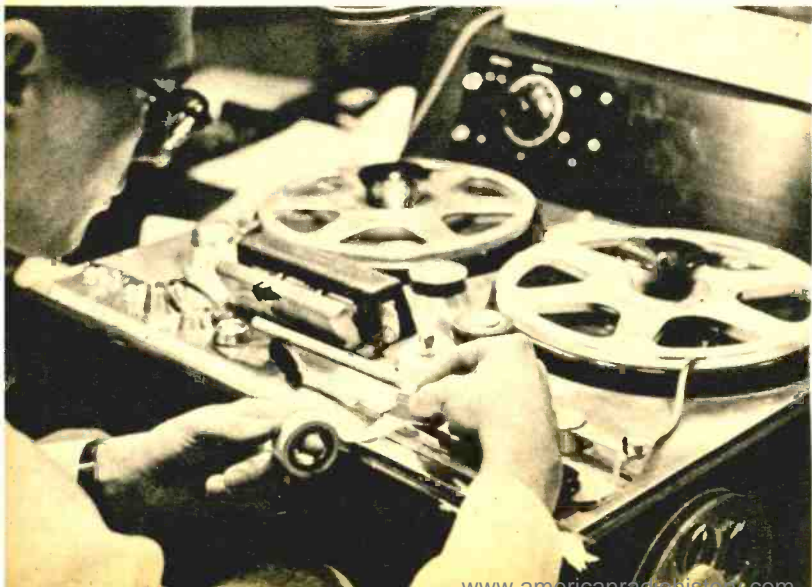
Cutting and splicing, listening; more cutting and splicing, more listening. These are the duties of the tape editor, a most important man in the recording business. (Photo taken in Columbia Records studio, N.Y.)
