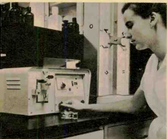
Chloridometer replaces old, slow chemical titration method of measuring chloride-ion content of blood serum with higher accuracy.
