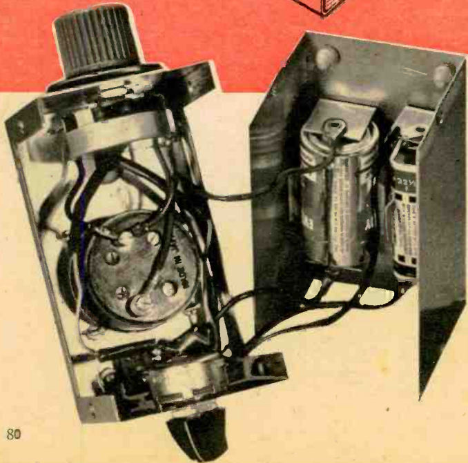
Tight quarters of case requires careful positioning of components. Note batteries tucked within cover.
