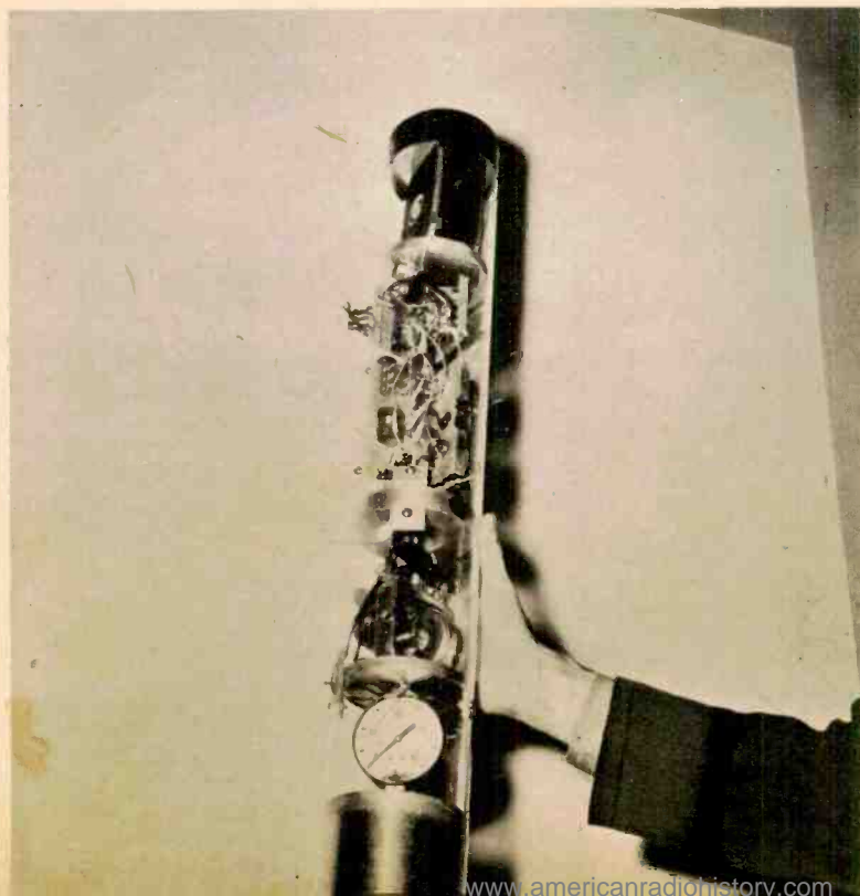
Part of instrument package of High Altitude Research Vehicle (HARVY) by Michael Tate, 16, of New York. Movie camera can be seen at top, pressurized chamber, bottom.
