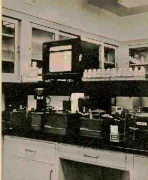
Auto-analyzer for blood plasma does three times as many samples as older methods, at five times the accuracy in same working time.
