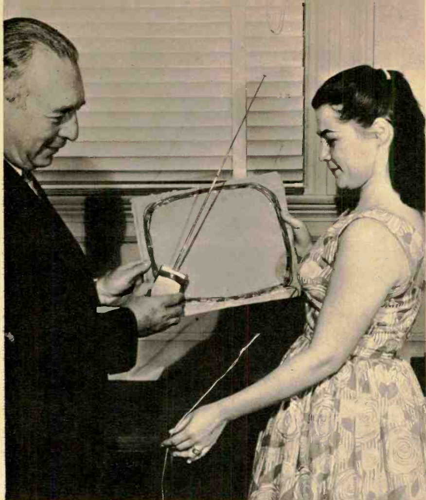
Novelty set performs well if held near induction loop of long-wire antenna (which may be hidden under counter) but works poorly away from it.
