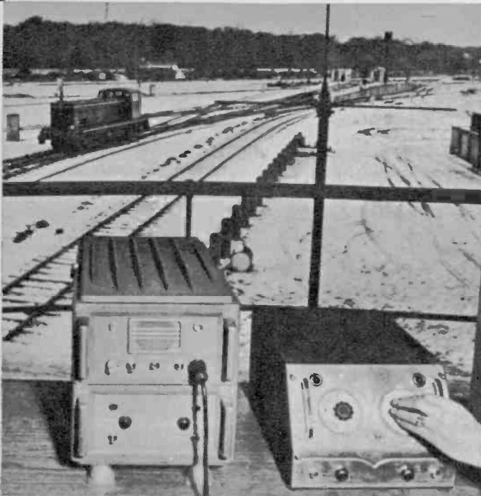
Paris would be a model rail-roader's paradise. French control setup shunts engines, couples and decouples trains, runs entire yard from single control tower. Standard type engines have nobody aboard.
