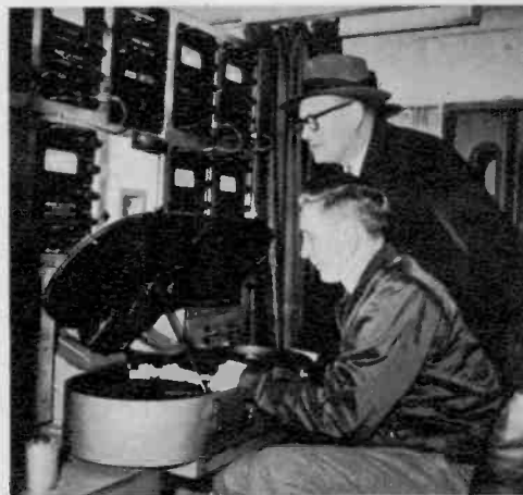
Technician on moving shop car inspects tracks with ultrasonic flaw detector. Method is more reliable as well as faster than visual check.
