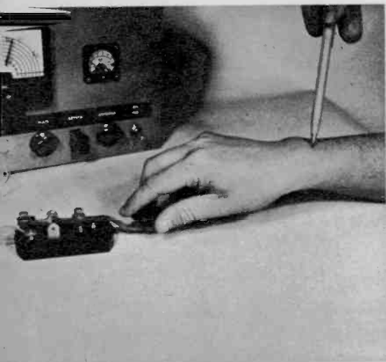
Proper key technique consists of grasping key gently and imparting an up-down wrist action.
