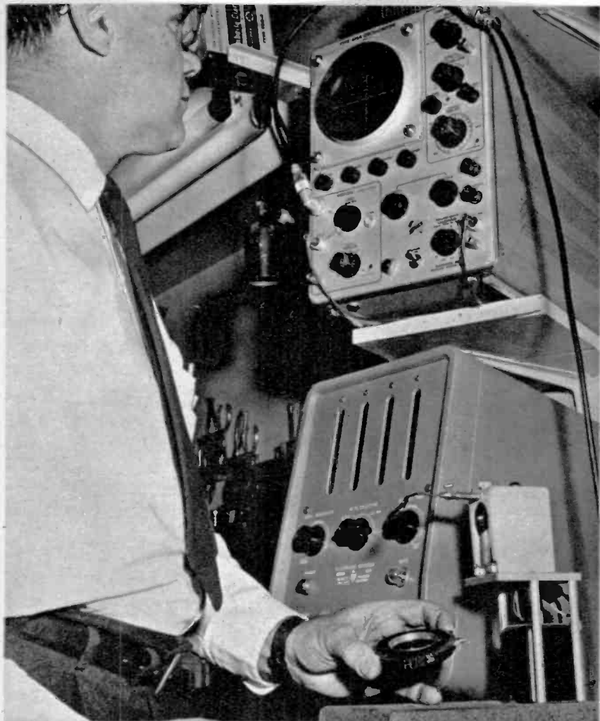
Photo-electronic consultant Irv Jacobson gets set to test lens shutter in his lab. Light passes through shutter to photocell (lower right) and is recorded on oscilloscope. This gives an accurate check on the speed of the shutter.
