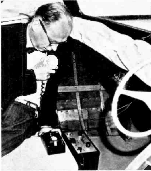
To check whether CB transmitter is putting out the maximum allowable signal, make use of a field strength meter such as one shown here.
