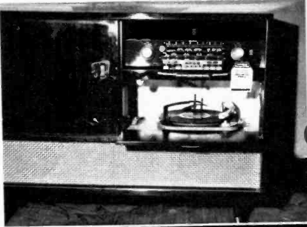
West German Grundig stereo consoles have elaborate tone and push-button controls and record storage space. Tuner is not adapted for multiplex, nor will it play AM-FM stereo.
