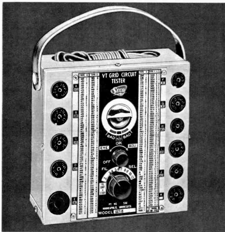
Fig. 4 shows another control grid emission tester. Features ten pre-wired sockets and an electron-ray tube indicators.
