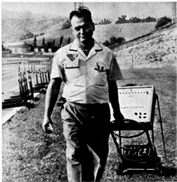
The control panel can be hauled around the track to wherever it is needed. Note 12-volt auto battery at bottom of special handcart. Starting panel also operates on 117-volt AC.
