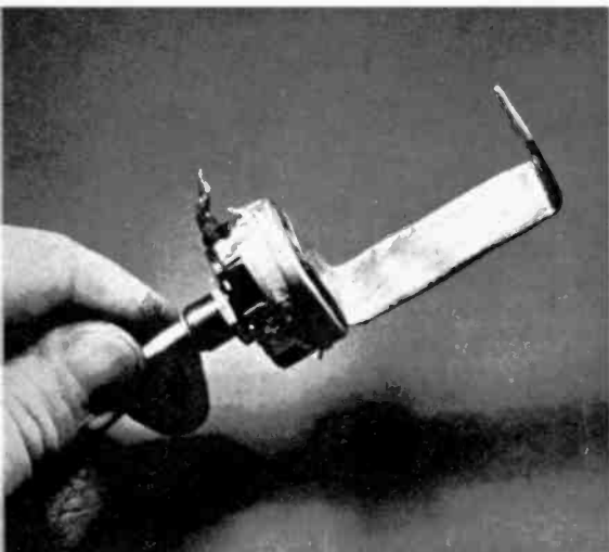
R4 has one end soldered to metal bracket preventing it from turning with vernier.
