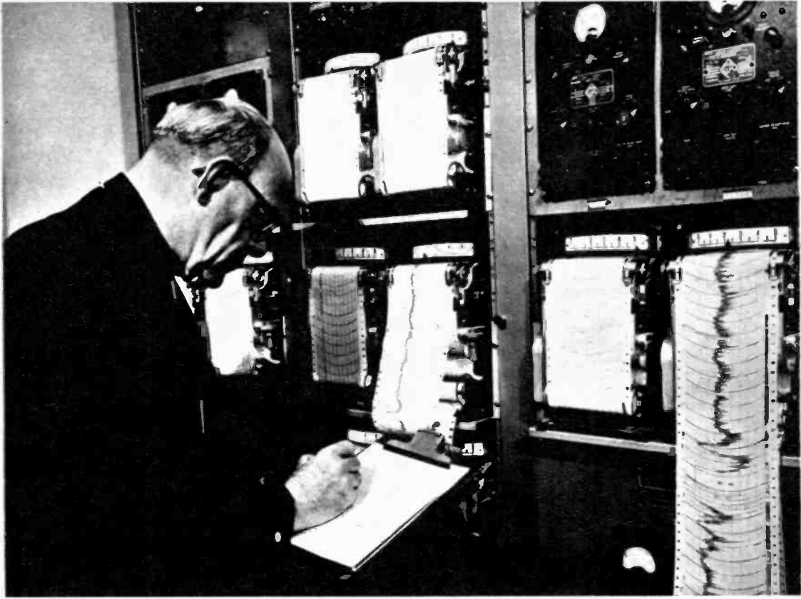
Records taken at Gunbarrel Hill radio observatory (Bureau of Standards) are of solar noise. This information helps predict propagation disturbances.
