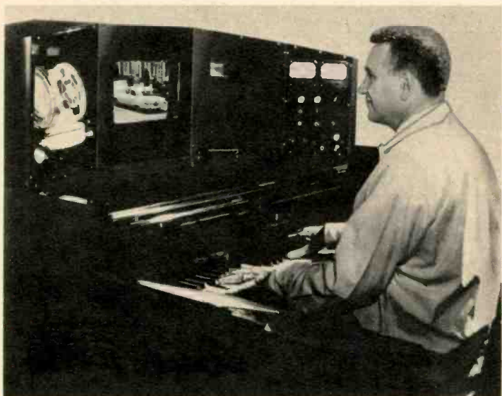
Movie-makers have brought electronics into the act also, with a closed circuit TV system for composing background music for sound tracks. Composer Raymond Scott sits at a "Videola", which includes a Blonder-Tongue Monitor TV receiver. A tape recorder at his left records his music; the TV monitor shows film for which it is intended; and at his right are push buttons for indicating film footage, volume meters, and selector buttons for watching the film and/or listening to the dialogue.
