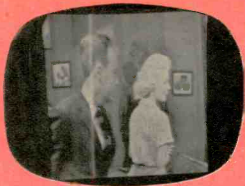
SMALL PICTURE, INSUFFICIENT HEIGHT AND WIDTH; Low voltage rect., damper, horiz. output.
