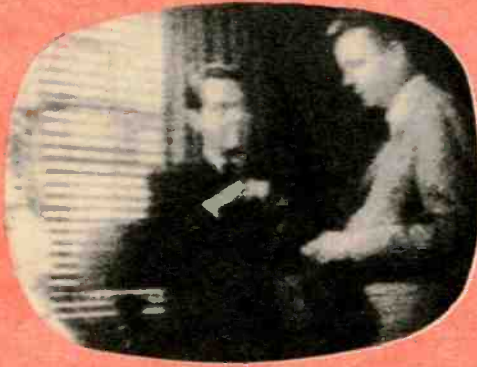
WEAK PICTURE WITH SNOW; RF amp., AGC. If picture is weak with no snow, check HF oscillator, mixer, video IF, video detector, video amp.
