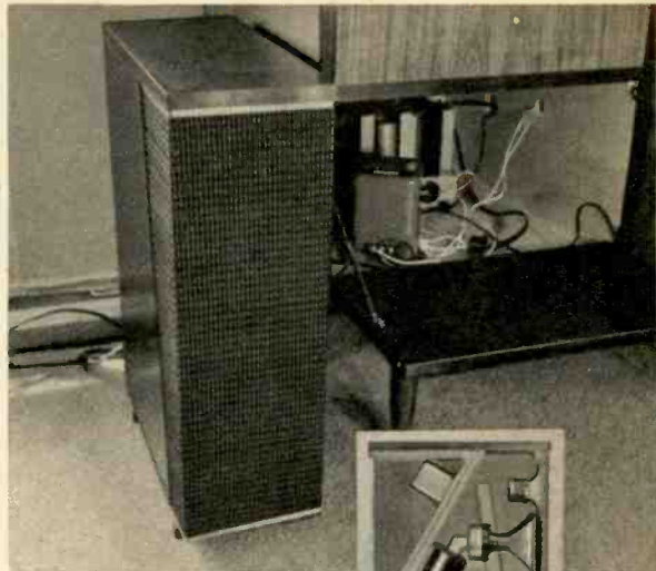
Electro-Voice Stereon speaker system contains only mid- and high-frequency horns, supplies directive range of hi-fi sound.
