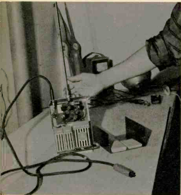
Bramco tone xmtr works CG rcvr. Keying lead with phone jack allows placement on car roof.
