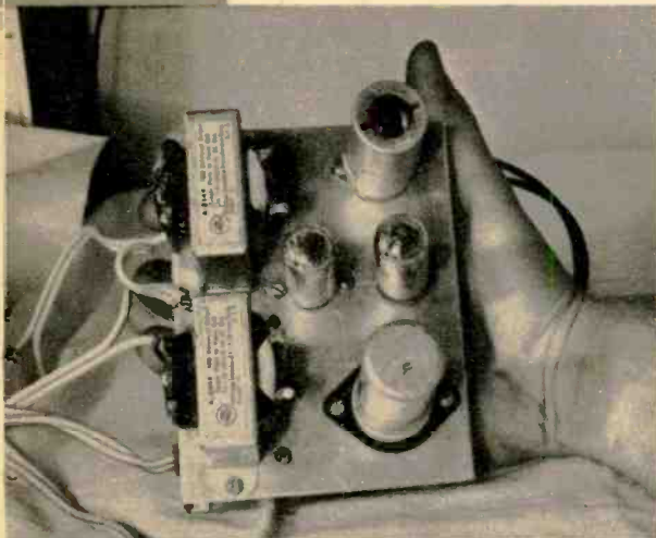
The additional parts visible on top of the amplifier chassis are two output transformers at left and the 50C5 output tubes, center. Right photo shows the dual control R11 and R12. On the chassis left to right are C3, V2, and V1.
