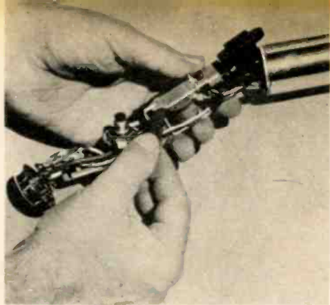
Relay points are cleaned with very fine grade of emery cloth. See text for adjusting process.
