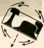
Jensen DS-100 speaker system has two woofers pointed down two mid- and high-range units that can be rotated toward the listener.
