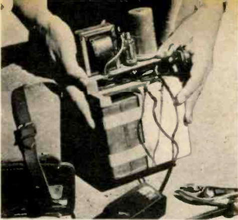
Bad condenser is replaced with a light wooden box (center right) to support the other parts.
