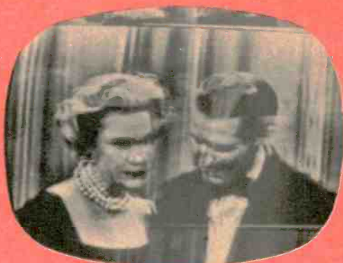
LOSS OF VERTICAL SYNCH; vertical oscillator.
