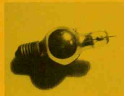
Fig. 8 Hot-cathode construction for mercury-vapor rectifier tubes.
