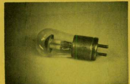
Fig. 25 The full-wave cold-cathode BH rectifier tube.
