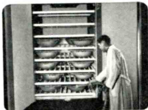
Drying ovens remove moisture from phosphor
