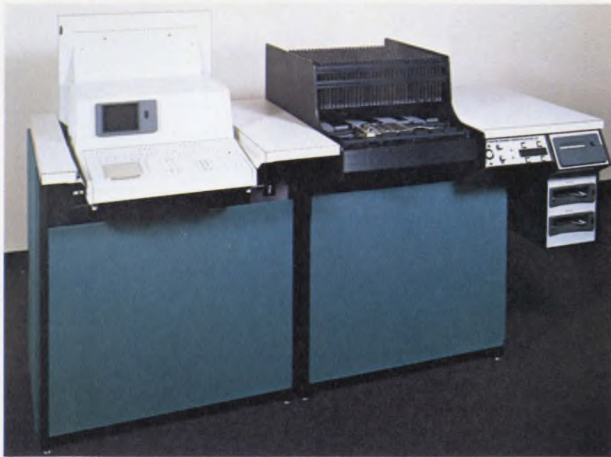
Rubber-tipped pressure rods hold PC boards in place on Teradyne's L529 tester. The system screens out workmanship errors before functional testing.
