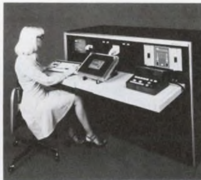
The lowest-cost in-circuit tester using a bed-of-nails fixture is Computer Automation's Mica 5000 system. Its price, as low as $30,000, is less than half that of some competitors.
