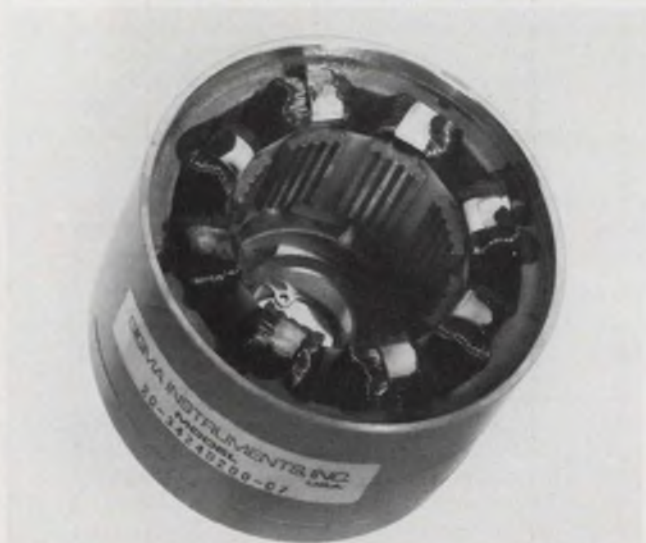
Permanent-magnet stepping motors contain stators with a number of wound poles. Each pole has several teeth as part of its flux distributing member.
