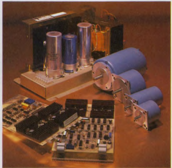
A stepper motor should be considered a system , not just a component. Electronic driving circuitry is needed and can significantly affect performance.
