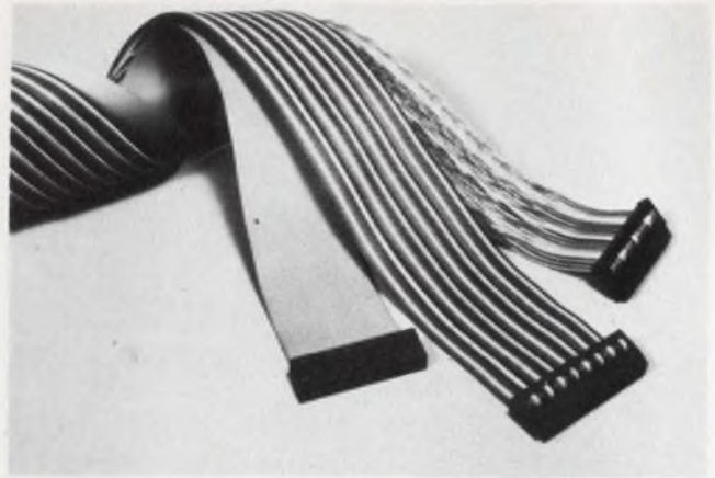
Twisted wires minimize crosstalk , but are difficult to terminate. By alternating twisted sections with flat sections, this cable from Alpha Wire Corp. (right cable) can be mass-terminated like other flat cables.
