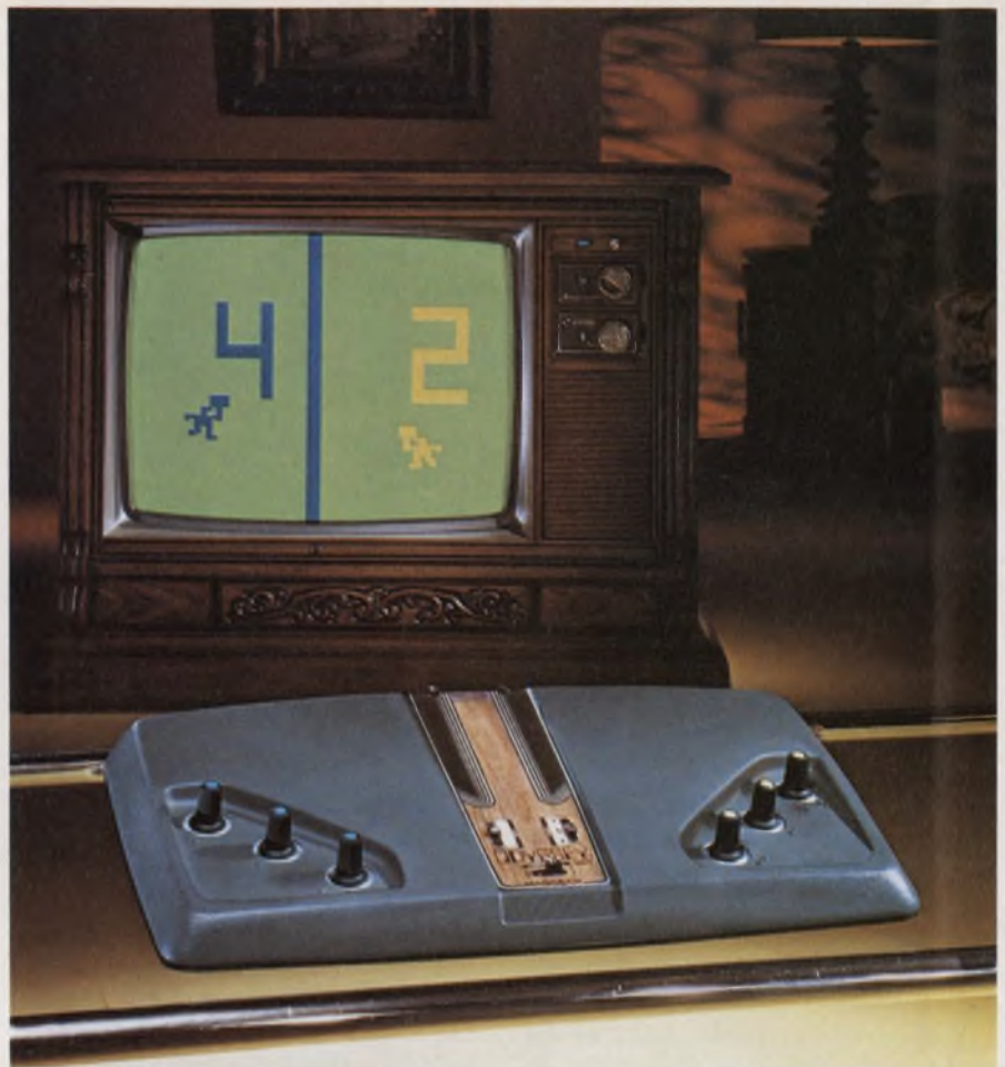
Four games are contained in this Odyssey 500 unit by Magnavox: Tennis, Hockey, Smash and Soccer. In these games—originated by Magnavox in 1972—the players are represented by on-screen figures.
