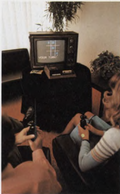
The first microprocessor-based video game to be marketed was this Fairchild Channel F system with programs in plug-in ROM cartridges.
