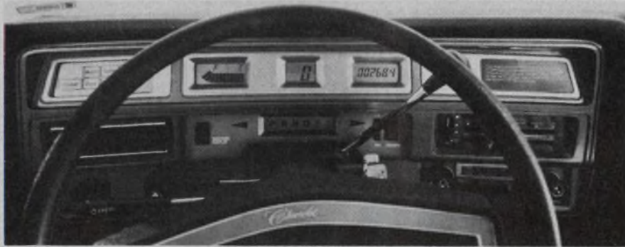
A liquid-crystal displays like this one may be used in future cars.
