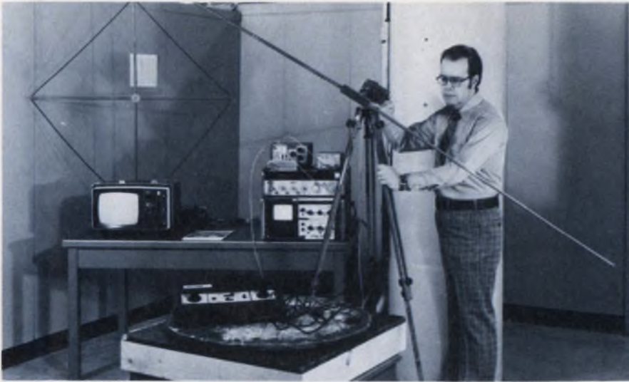
Making EMI/RFI measurements to check the levels of radiation from TV games is only part of the problem of getting video games to pass FCC standards. Here, Dan Norton at Sanders Associates checks on a design fix.
