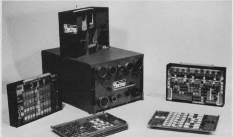
An airborne computer, dubbed the AN/AYK-14, has been developed for the Navy by CDC. The heart of the unit is the AMD 2901 microprocessor.
