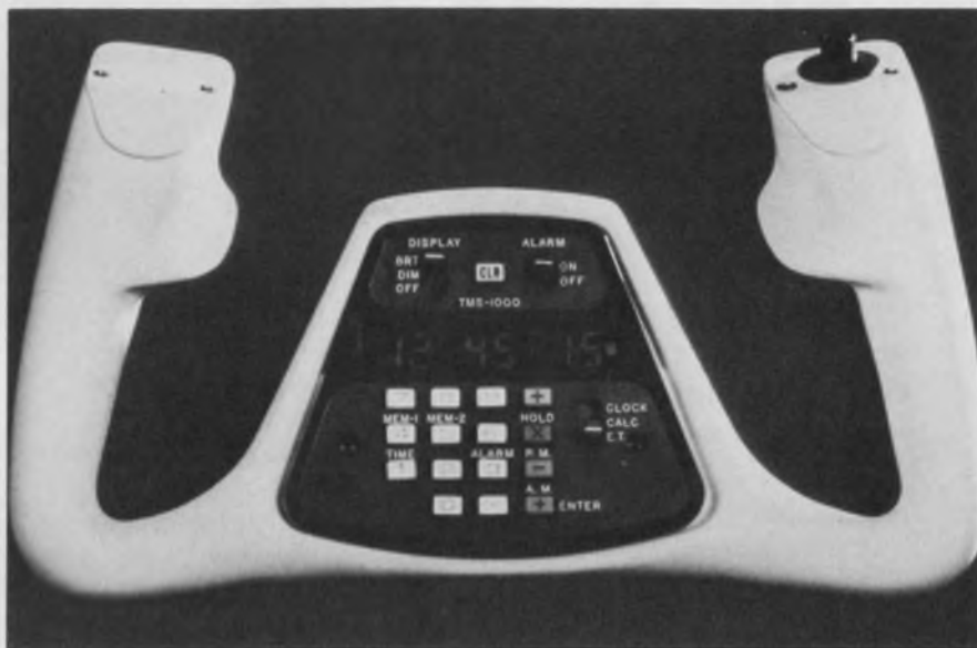
A two-chip MOS calculator and clock-timer reduces pilot's in-flight workload. The TMS-1000 by Martin Avionics, requires tight packaging, enhancement of the LED display, and elimination of EMI.
