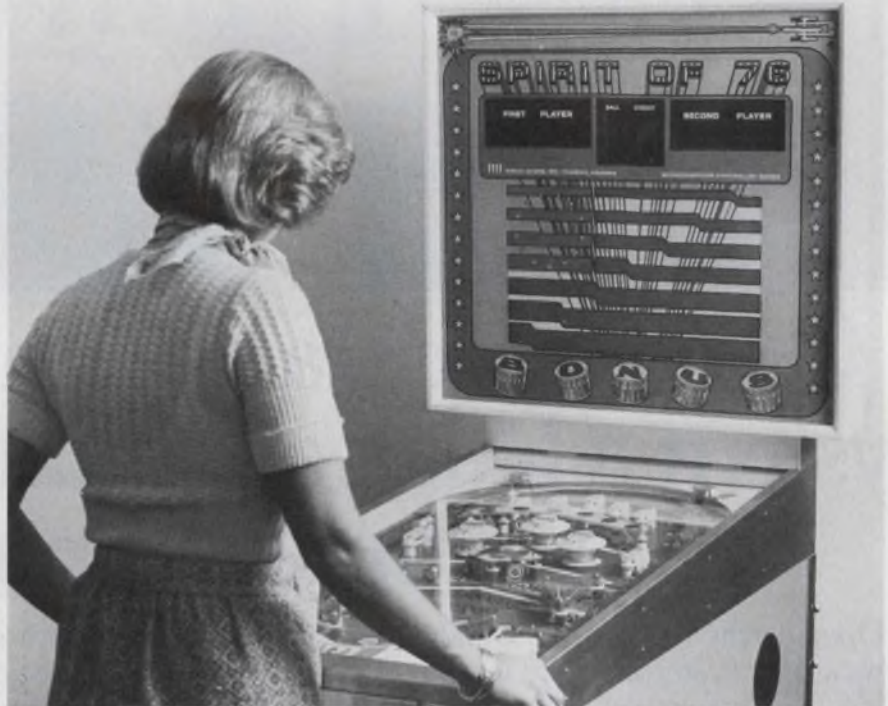
Microcomputer control of a pinball machine makes troubleshooting simple. The Mirco Games unit uses only 1/10 the power of regular machines.
