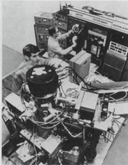
EBES electron beam exposure system from Bell Labs increases accuracy and efficiency of IC production.
