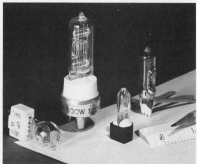
Special, highly stable ceramic-like adhesive can perform satisfactorily up to 2200 C. Here a Sauereisen inorganic cement is used for stable alignment of lamps operating up to 330 C. From left to right: a film projector lamp, a flash bulb and an aircraft warning light. At far right, external leads of mercury switch are sealed.
