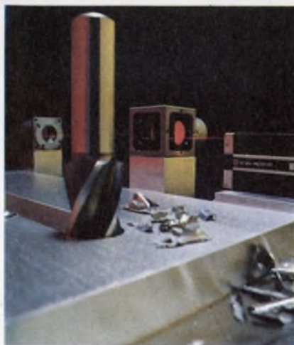
Machine-tool positioning is easy with the Hewlett-Packard 5501A Laser Transducer System. The system uses a two-frequency laser head and interferometric optics for precise linear displacement measurements.
