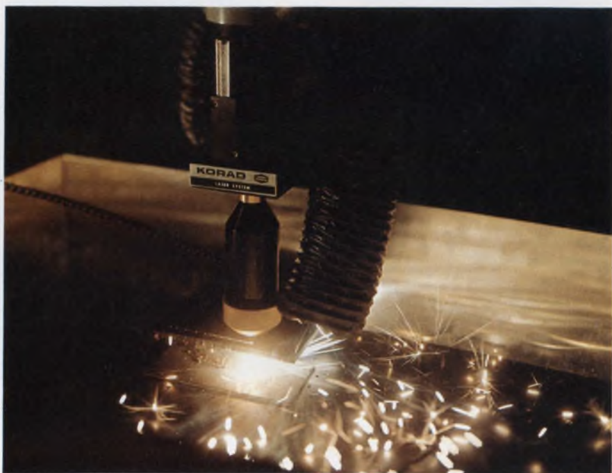
This Q-switched YAG laser, from Korad, is cutting through 1/4-in. thick titanium. YAG lasers are also being tested for communications.
