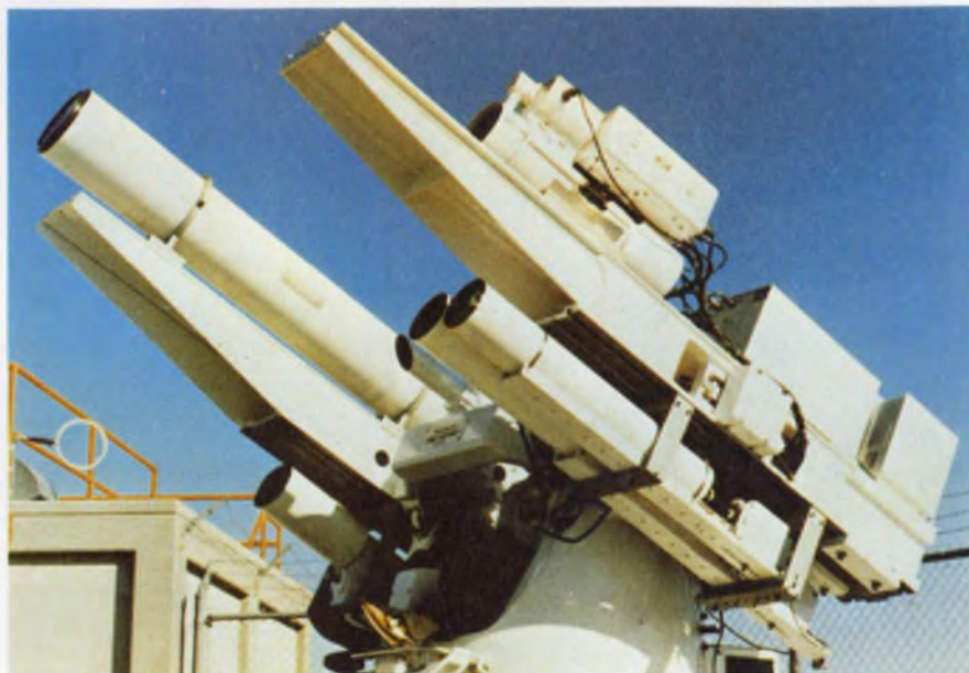
Like radar, lasers can be used to track aircraft and missiles. However, the lack of ground clutter with systems like this Nd:YAG laser tracker from GTE Sylvania allows low-flying vehicles to be tracked with great accuracy.
