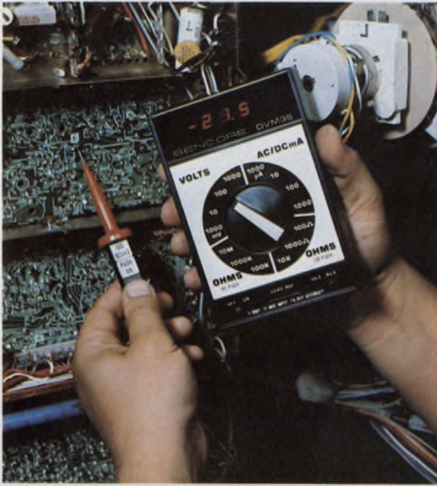
Pocket portables are getting smaller. Sencore's DVM 35 illustrates the trend toward lighter and more compact meters. The 3-digit 35 sells for only $124.
