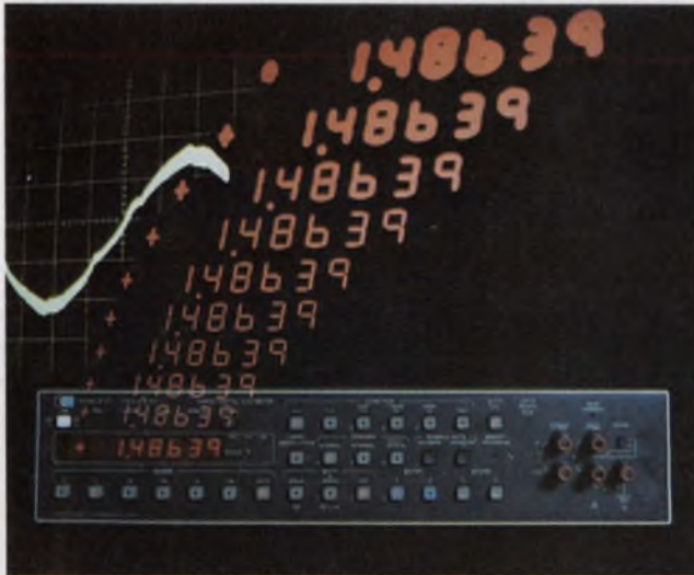
With internal \mu Ps and memories, systems DMMs are growing in sophistication. This Hewlett-Packard unit is the first to offer a removable reference module.
