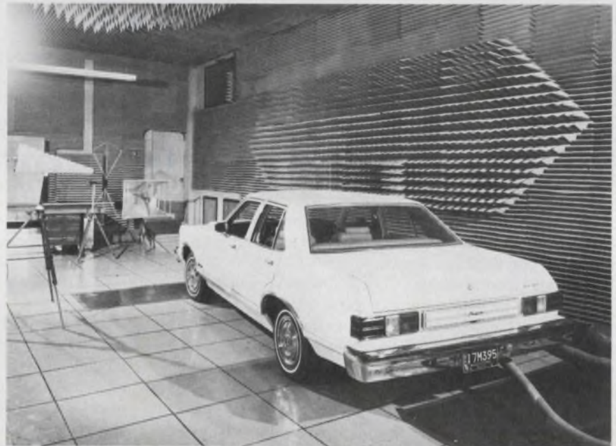
Vehicles are isolated from external environmental noise to define and reduce their EMI in the anechoic chamber at Aeronutronics Ford, Palo Alto, CA. The EMI is pin-pointed and measured from 20 to 1000 MHz.
