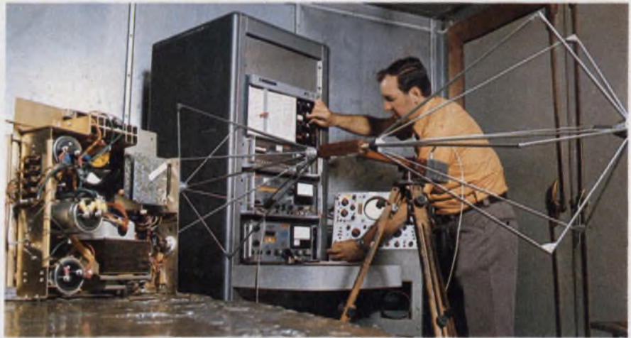
Radiated interference from a display-terminal power supply being measured for a customer at Sanders Associates, Nashua, NH, electromagnetic-compatibility test facility. Measurements are being made between 20 and 200 MHz.
