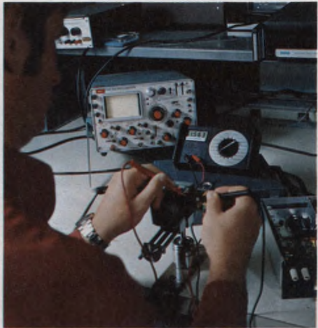
This DMM lives up to the name "multimeter." The unit is also a 27-MHz counter. Battery operation lets you take the Valhalla 4440 into the field.
