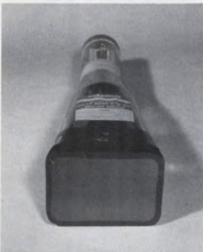
Rectangular face fiber-optic CRT is used for direct photo-recording in electro-medical instrumentation. It's available from M-O Valve Co. Ltd., London.
