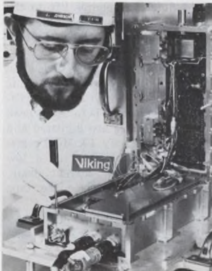
The Viking Lander's 10-lb uhf radio is used for high data rate traffic from the surface to the Orbiter, where it is converted to S band.
