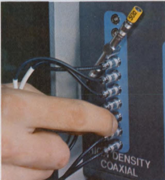
To install push-on connectors such as these Lemo self-locking types, you don't require all-around finger space to twist or turn; thus, many can be closely spaced in-line to save panel room.
