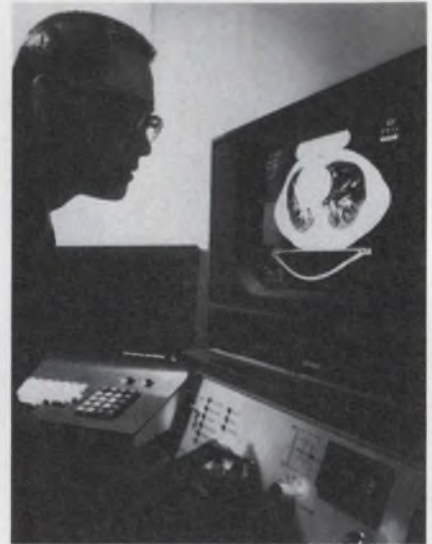
This CT scanner X-ray image, showing the vascular patterns of a human lung, was taken in less than 5 s by GE's new whole-body scanner.
