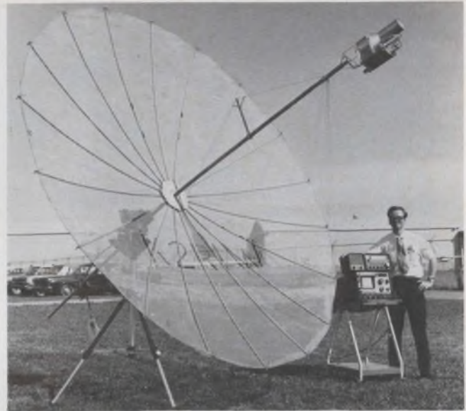
Voice signals from Apollo 15 and 16 astronauts on the moon, were received by radio amateur Richard Knadle using his home-made $42 parabolic antenna. Transmitter power on the moon was only 13 W.
