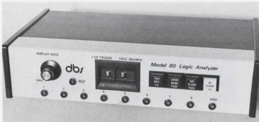
A stand-alone analyzer from Digital Broadcast Systems delivers a multiplexed signal to an external scope.
