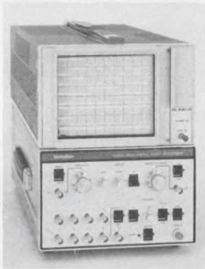
One of the first analyzers on the market is still a best seller. The unit is Biomation's 810-D digital logic recorder.
