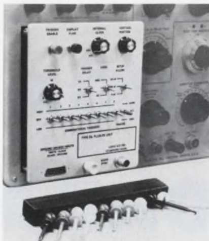
Another form analyzers take is the scope plug-in format. This one is from Logic Aid Inc.
