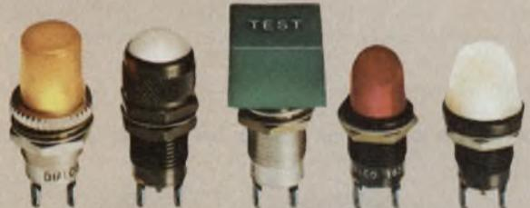
**INCANDESCENT OR NEON SUB-MINIATURE INDICATORS**—Meet or exceed MIL-L-3661. Mounts in 15/32", 1/2" or 17/32" clearance holes. Incandescent for 1.35-28V; neon has patented built-in current limiting resistor. Choice of cylindrical, faceted, convex, flat, square and round lens shapes, finishes, legends. Stocked by local distributors.
