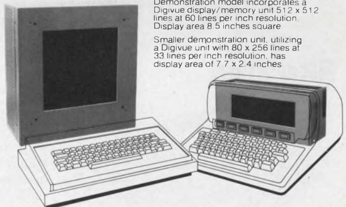
Demonstration model incorporates a Digivue display/memory unit 512 x 512 lines at 60 lines per inch resolution. Display area 8.5 inches square
