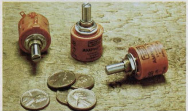
Miniature panel-mounting potentiometers by Amphenol, such as these Model 4201Bs, can handle several watts of power and provide multiturn resolution.
