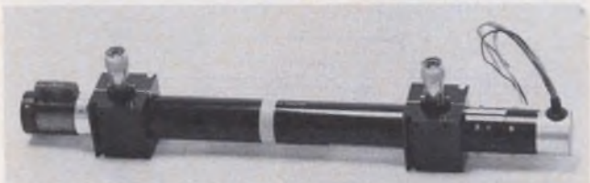
6. A transpiration cooler is easily retrofitted to a traveling-wave tube. Its performance curve is similar to that of the cooler shown in Fig. 5.
