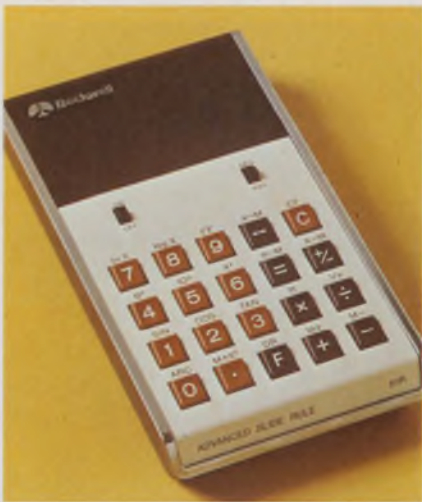
Capabilities of this eight-digit, floating-point calculator, the Rockwell 61R, are duplicated in a sizable number of other machines.
