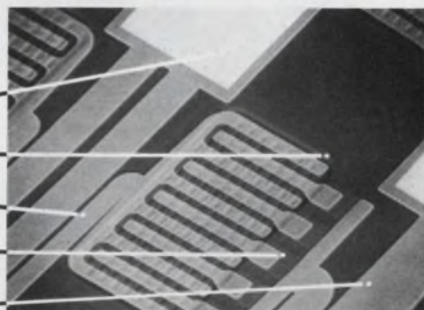
ONE OF THE 48 INDIVIDUAL CELLS ON THE 60 x 165 MIL MRF306 CHIP
