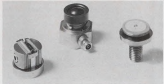
Piezoelectric accelerometers (shown without their cases) use one or two slices of piezo material.
