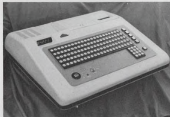
Staid Corporation's Datacash —a microprocessor-based point-of-sale terminal for restaurants—keeps an inventory of every key strike.
