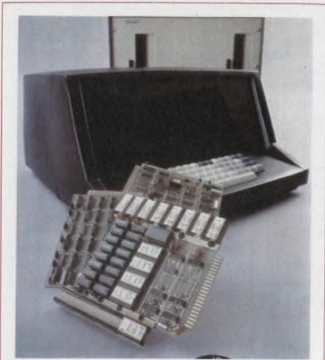
Dasyn's 101 universal terminal uses single-bus architecture and an Intel 8008 CPU to provide considerable flexibility. A variety of memory boards and I/O interface boards and peripheral controller boards can be plugged into the bus.
