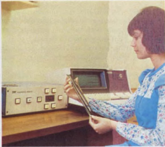
Holographic data retrieval unit from IRW is used to read data stored on 35 mm film. A holographic recorder is used to store data.
