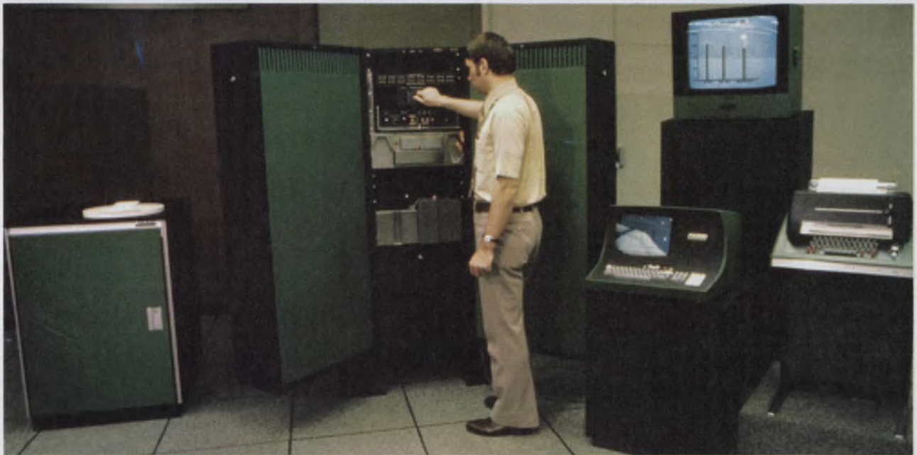
A Western Electric plant in Massachusetts uses a DEC PDP-8 minicomputer to monitor and control several coil-winding stations. The stations are
