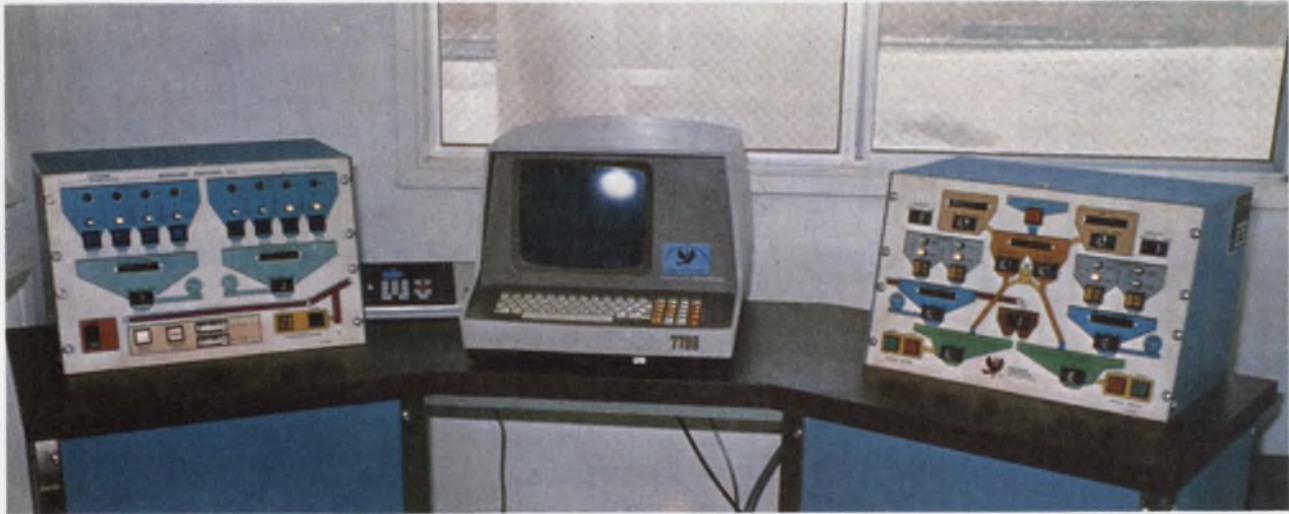
Automated batching systems by Phoenix Engineers are built around Cincinnati Milacron 8000-series
