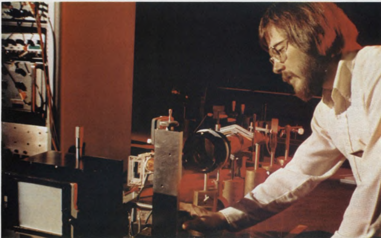
Optical memories like this one from Sperry Univac are being designed to store up to 10^{10} bits of in-
