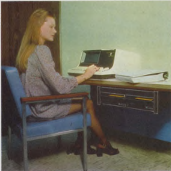
Kennedy Data Systems' KDS-28 contains a pair of Century Data Systems floppy-disc drives and a controller. Interface electronics are included to mate the disc drives to Datapoint terminals.
