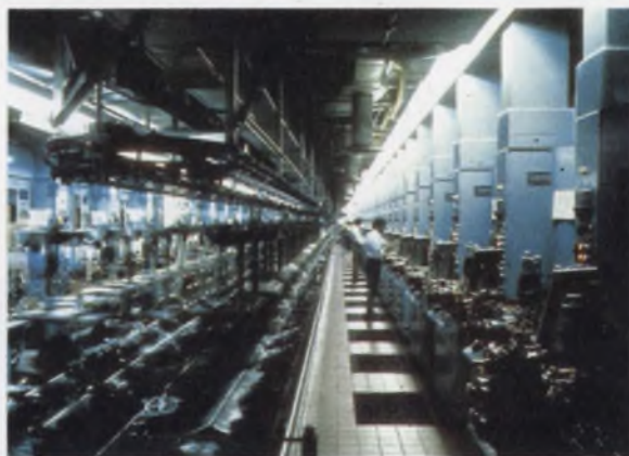
Rows of carburetor-flow test stands are individually controlled by SPC-16 minicomputers from General Automation. Groups of 31 stands report to an IBM System/7 supervisory computer, which, in turn, acts as a data concentrator for a 370/145. This hierarchical computer organization operates at the Rochester Products Div. of General Motors.
