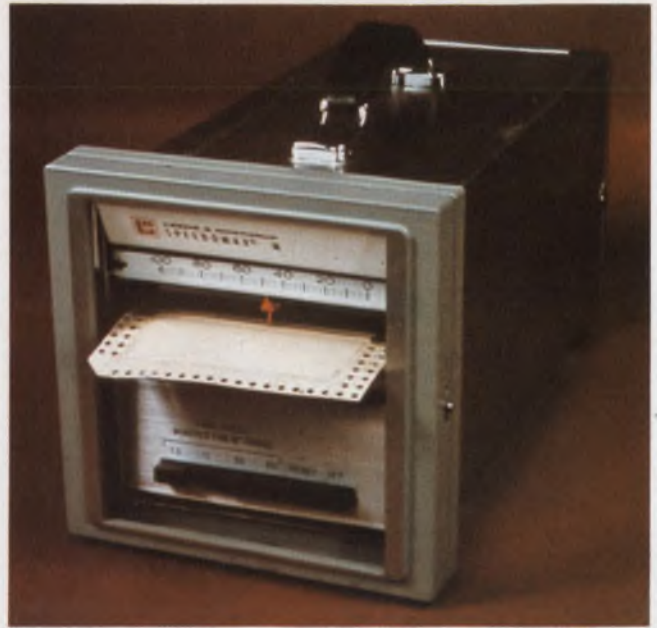
A novel card-chart recorder from Leeds & Northrup allows analog information to be recorded on cards for easy filing and later retrieval.
