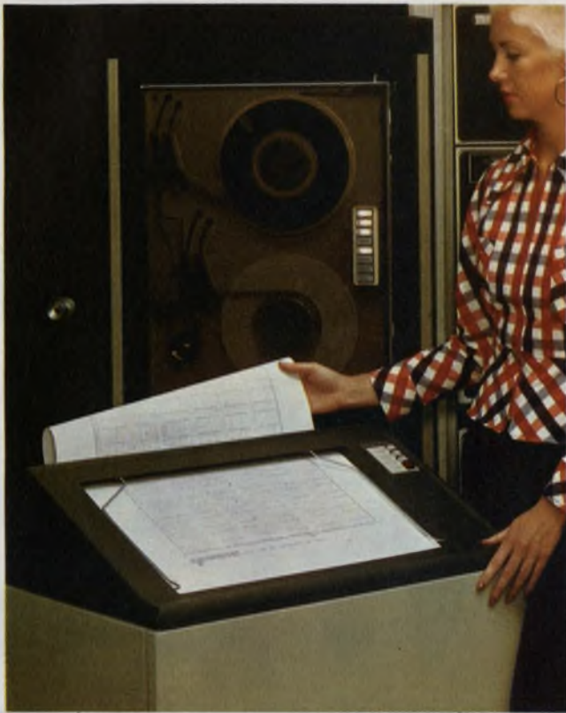
Matrix electrostatic writing is the recording technique used in the Versatec printer/plotter. A special electrographic paper must be used with these units.
