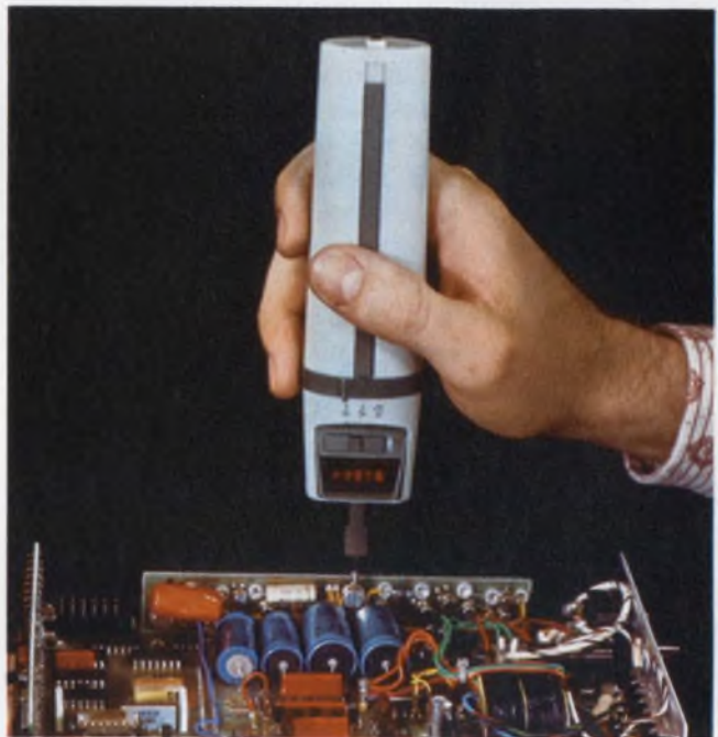
The HP-970A takes top honors for being the smallest DMM available. It measures ac/dc volts and ohms, but still fits into a shirt pocket.
