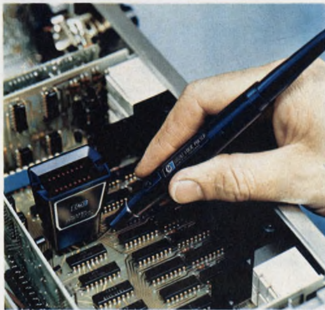
Logic pulsers and clips, like these from HP, are used to provide a stimulus to a logic device and indicate its response to that stimulus.
