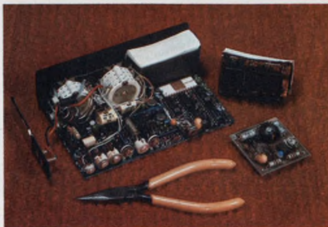
A flexible assembly for the indicator circuit and rigid boards for the rest allows Data Precision's Model 245 DMM to pack many parts in a small space.
