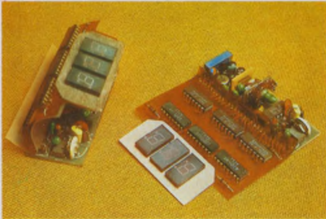
The flexible PC assembly in Analogic's Model 2530 DPM can be unrolled for convenient servicing, and the unit remains operational.
