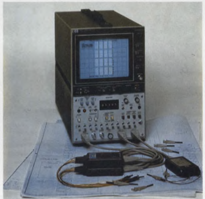
The 1601L Logic State Analyzer from HP is the newest arrival on the digital test equipment scene. It allows designers to analyze parallel data streams and displays information in truth table format.
