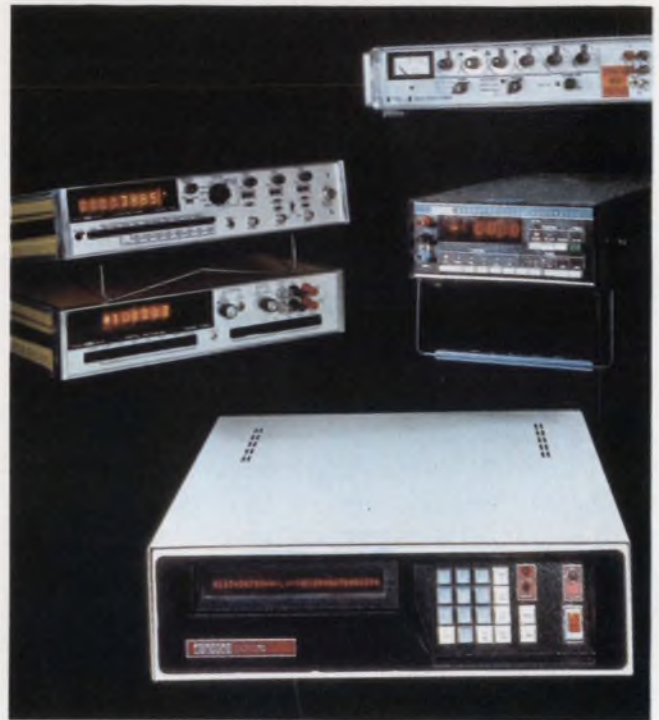
TTL-compatible instruments become a stand-alone system when connected to Digital Equipment Corp.'s intelligent controller—the PDM70. Plug-in interface modules convert instrument responses to bit-serial ASCII for use on the internal controller busses. A user-entered stored program enables data transfer between instruments. A special module permits communication with ASCII-serial computer ports at rates up to 39,000 baud. Thus any computer that communicates with a TTY can also process instrument data.
