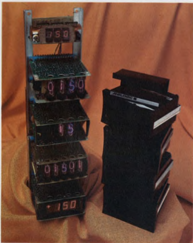
LEDs, Nixie neon tubes and seven-segment Sperry tubes are used by Analogic in its line of DPMs. The displays have 2-1/2 to 4-3/4 digits.
