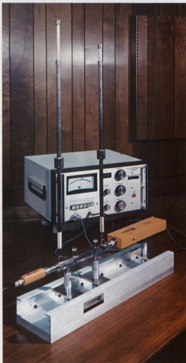
Designed specifically for calibrating microwave noise sources, the Ailtech 82 requires only 28 V dc at less than 15 mA. Earlier devices were bulky and power hungry.
