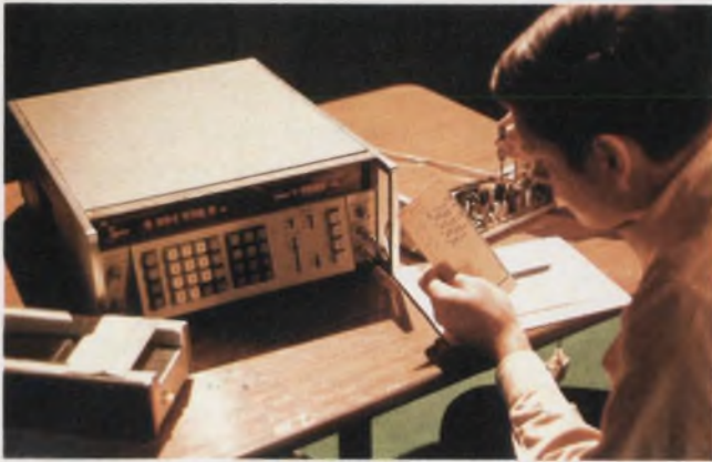
Instruments and devices equipped with HP's ASCII bus can be plugged together to make up a system. The programming device in this case is the HP 3260A marked-card programmer, which acts as the controller for the 3330A programmable frequency synthesizers.
