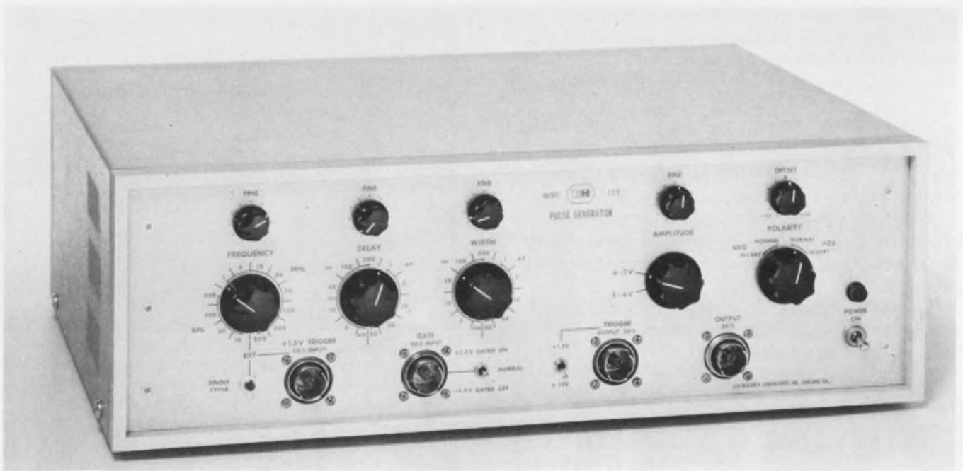
A 500-MHz repetition rate and transition times of 500 ps makes E-H Research Laboratories' Model 129
