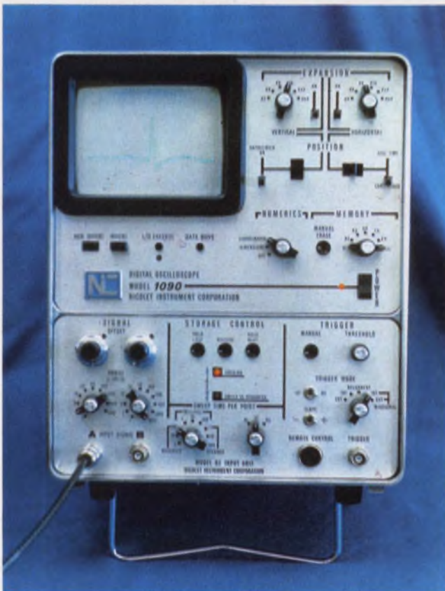
The Digital Storage Scope from Nicolet features a 12-bit resolution transient recorder and a CRT display. The bandwidth of the 1090 scope is 100 kHz.
