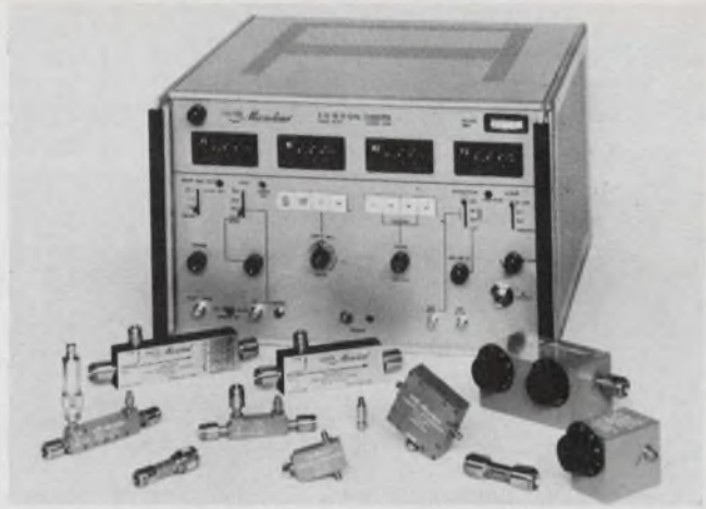
Narda Microwave's 9530 sweep generator covers 2 to 18 GHz in one sweep. Start, stop and marker frequencies are set by digital thumbwheel switches.
