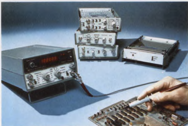
Some modular instruments are stacked horizontally. Hewlett-Packard's 5300-A modular measuring system snaps together in vertical sections.
