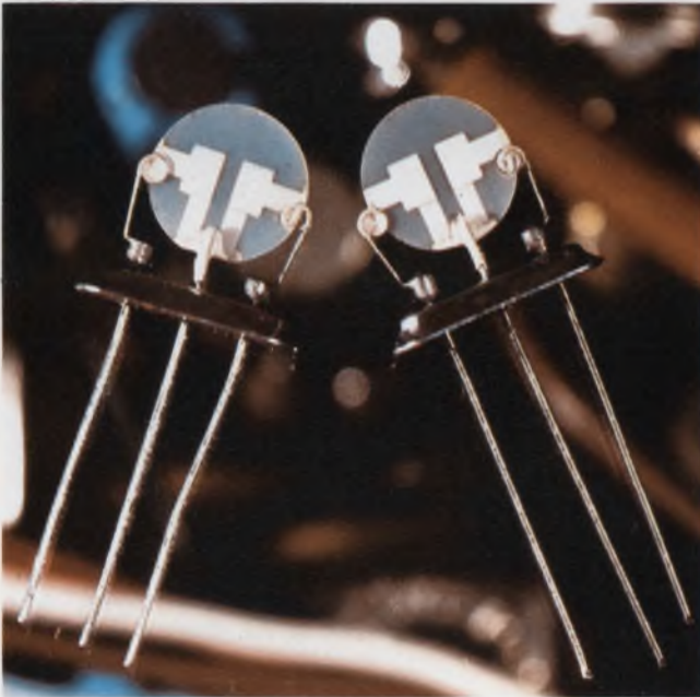
These two-pole, 21.4-MHz monolithic filters by Piezo Technology are ultraminiature. Four, six and eight-pole filters are made using multiple two-pole units.
