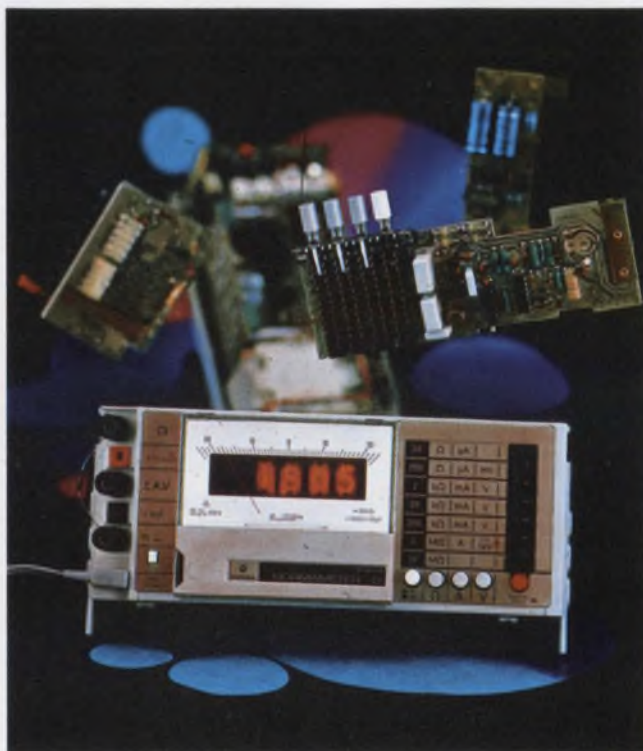
An unusual instrument is the Normameter D, marketed by the General Rand Corp. The 1999-count unit also features a zero-centered, analog meter movement.
