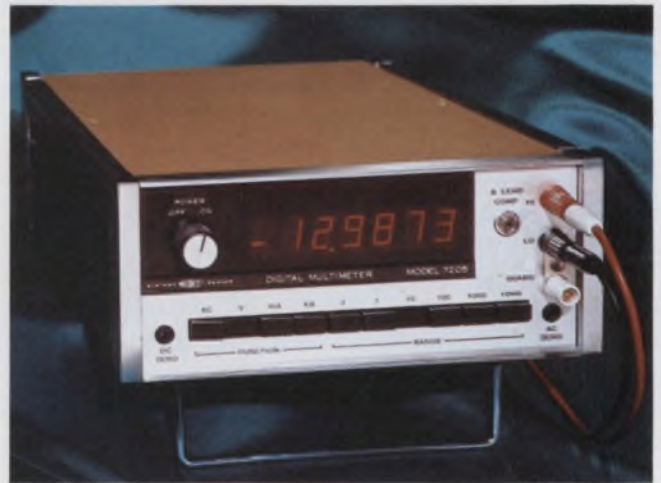
Systron-Donner's 7205 is a 130,000-count unit that features lead compensation on the ohms function.
