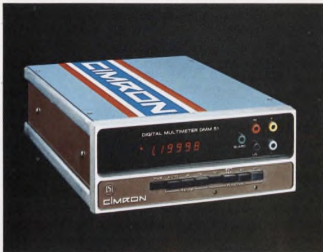
Lear-Siegler/Cimron's DMM-51 features ratio, four-wire ohms, autoranging and BCD data outputs.
