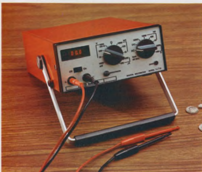
A new entry in the portable DMM derby is Ballantine's 3A-24, a 1200-count unit priced under $200.
