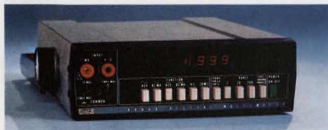
Fluke's 8000A—the first to use both analog and digital LSI chips. Featured are a high-impact case, overload protection and a weight of less than 3 pounds.
