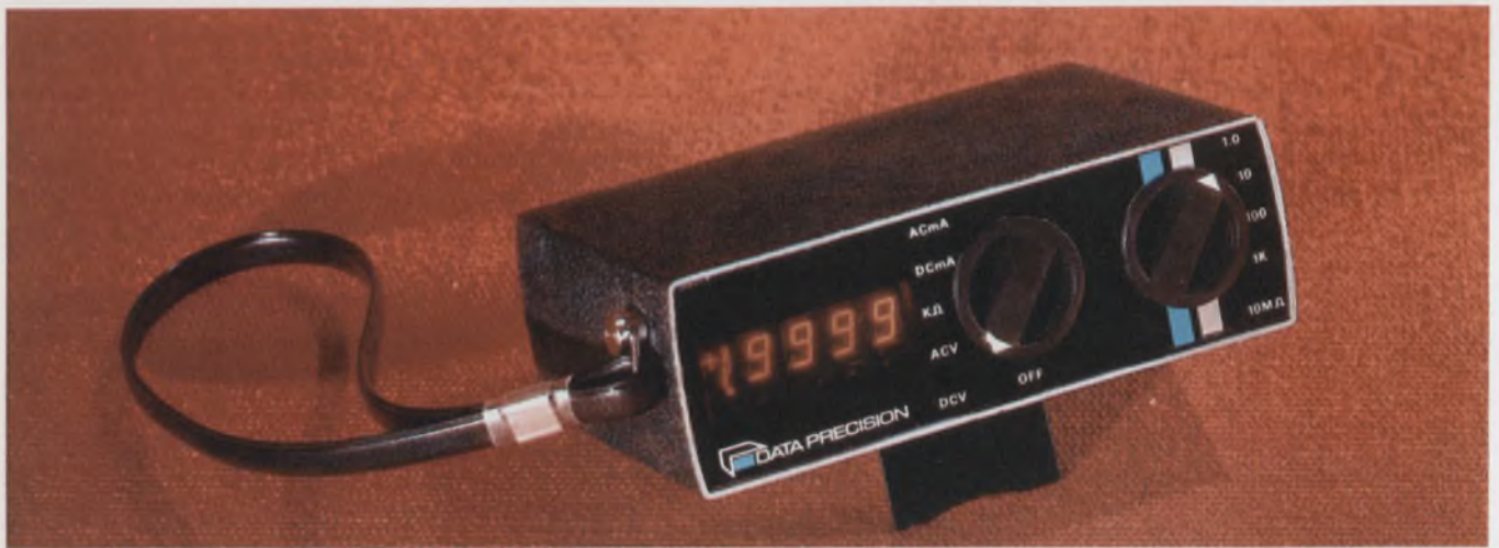
This pocket-sized midget is manufactured by Data Precision. The Model 245 weighs 1.3 pounds, counts to
