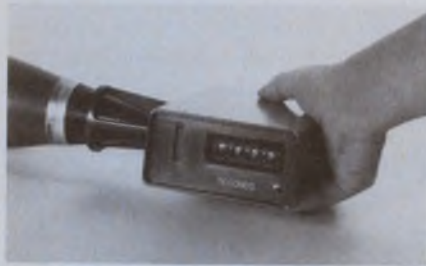
Timing information is entered into the MNOS memory in a new electronic fuze.
