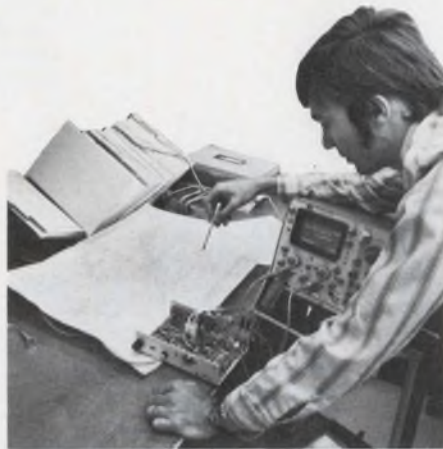
The 1710A scope is fast enough to test ECL, as shown here.
