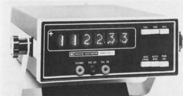
Non-Linear Systems' MX-1 counts to 119,999, autoranges and measures volts, ohms and ratio.
