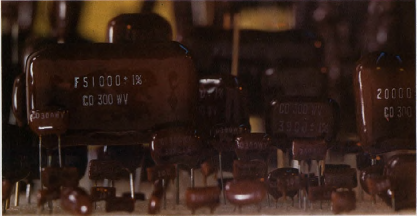
12. Dipped silvered mica-dielectric capacitors, such as Cornell-Dubilier's CD units, provide more capacitance in
