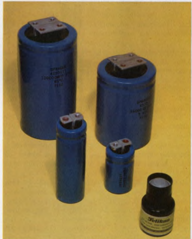
13. Sprague's stacked-foil, aluminum electrolytic is a good example of a functional improvement in a conventional passive components. Internal impedance is reduced to below 0.001 \Omega and inductance to less than 2 nH—well below most other electrolytic capacitors.
