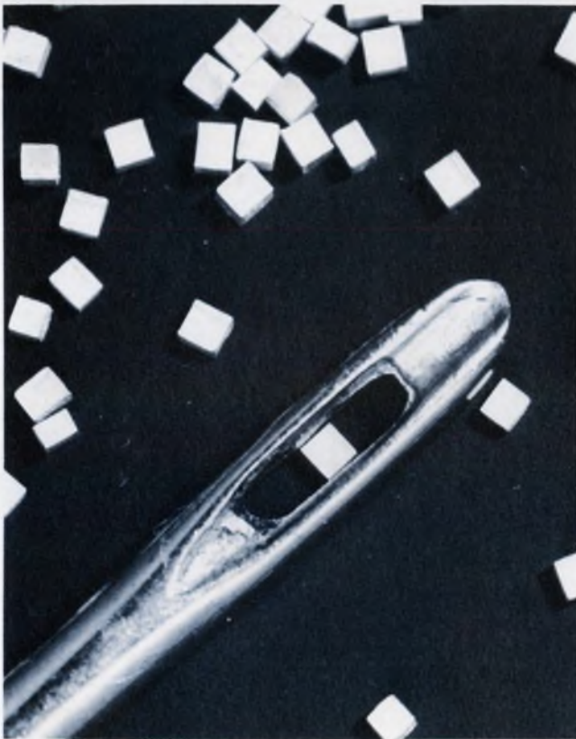
1. Chip components, such as American Technical Ceramics' rf capacitors, are the passive-component manufacturers' answer to IC-sized hybrid circuits.
