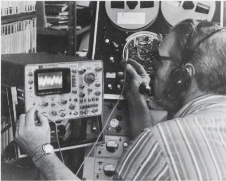
Here, a 1703A storage scope is used to check the audio circuits in a videotape machine
