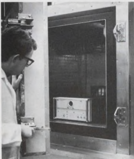
HP cesium beam standards undergo extensive environmental testing. Here, one is being tested at high altitude and high and low temperatures.
