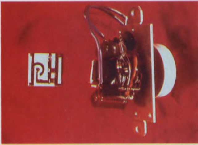
Electronic switching action is given by screen-printed and air-fired Tyox by Du Pont. The material is used in light dimmers and, here, as a switch in a thermostat.
