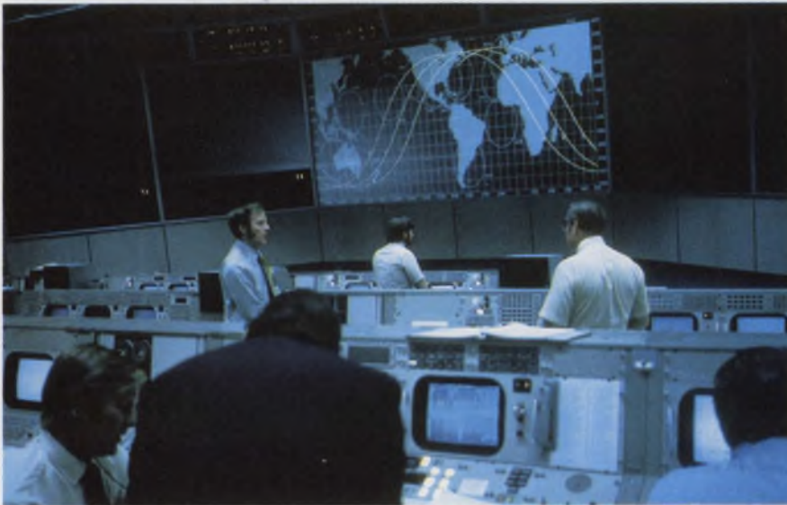
A new mission control center has been set up for Skylab at the space center near Houston. Information goes directly from digital data to a CRT display. The equipment occupies a fourth the space of Apollo's system.
