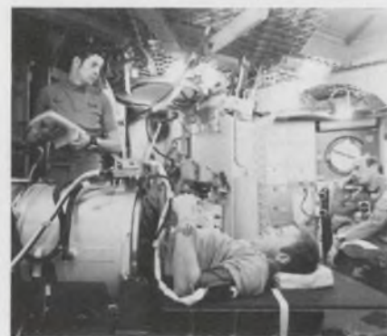
Astronaut Paul J. Weitz lies in the lower-body, negative-pressure device to measure loss of cardiovascular reflex in space. Astronaut Joseph P. Kerwin is standing, and Charles Conrad Jr. is seated.
