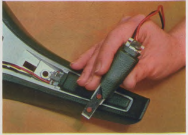
Pressing a new conductive elastomer in this steering-wheel button causes the horn to sound. The material, Pressex, has positive switching characteristics.
