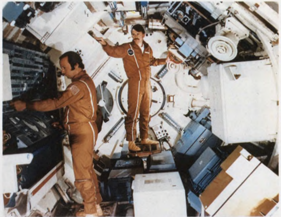
The workshop is a modified second-stage Saturn launch vehicle, 48 feet long and 22 feet in diameter, with 9550 cubic feet of living space; Apollo had 366. The console, at left, monitors the Apollo Telescope Mount's eight telescopes.
