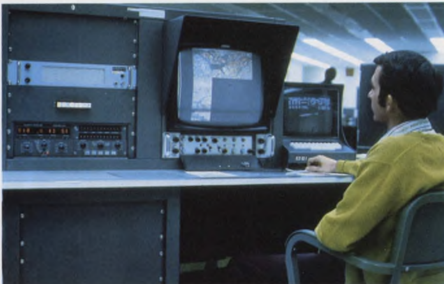
The readout for the earth-resources data from Skylab will be presented on this CRT in any of 512 shades of "pseudo color" arbitrarily assigned to different sensors to make particular features stand out.
