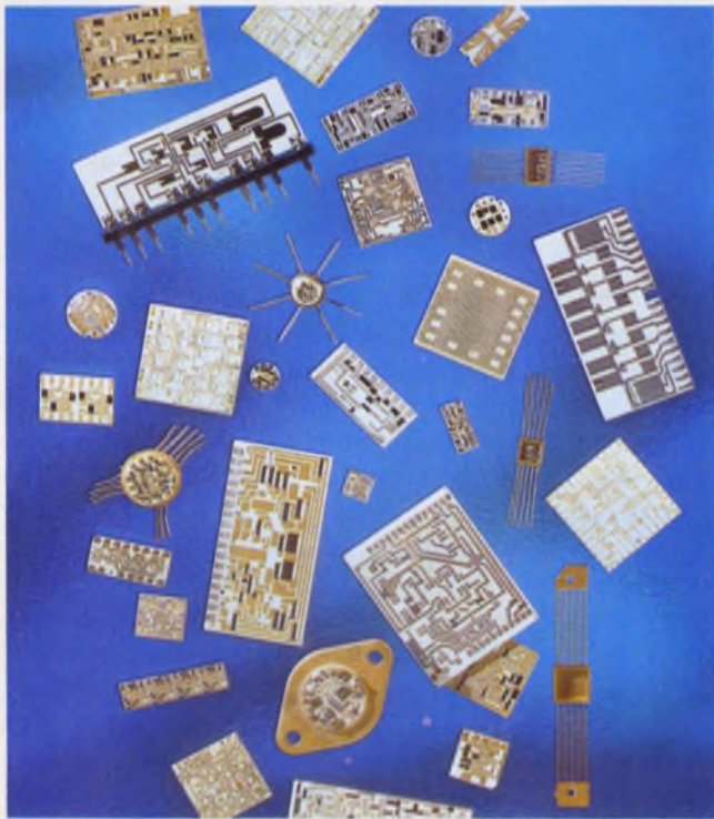
Use of thick-film circuitry is expanding. These samples from Sel Rex show a variety of microcircuits that were fabricated with thick-film compounds.
