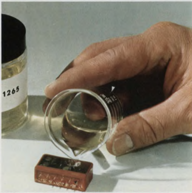
Epoxy compounds make up most of the potting materials. Components potted with this flexible epoxy gel, by Emerson & Cuming, can be dug out, replaced and repotted.
