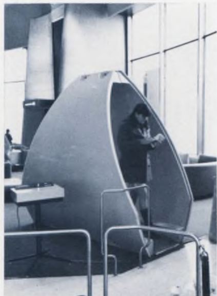
Metor weapons detector employs a two-part coil system embedded in a walk-through shell. One part is a transmitter producing an electromagnetic field, the other is a two-piece receiver coil. A phase discriminator measures the electrical core loss to determine the presence of weapons.
