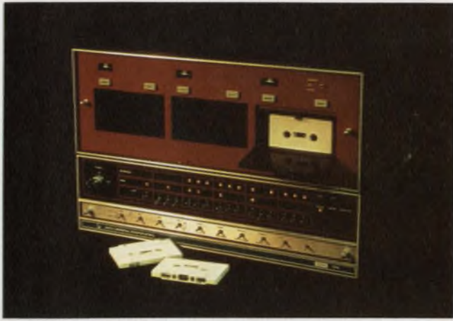
Data General has packaged three transports in a single package for use as a peripheral with its Nova minicomputers. The transports are of a reel-to-reel type with constant reel speed but variable tape velocity. Read-after-write recording heads are standard on this drive. An unusual encoding scheme avoids an extra clock track.
