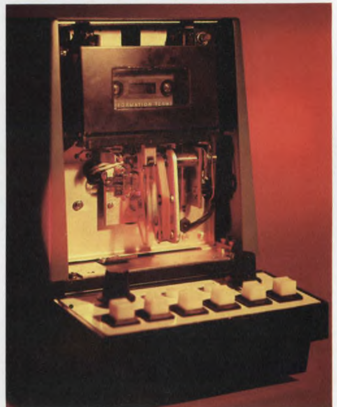
Bell & Howell's model 410 digital cassette decoder pulls tape out of the cassette in order to wrap it around a large capstan. This allows much more precise tape control than is possible with the small capstans that many other manufacturers use.
