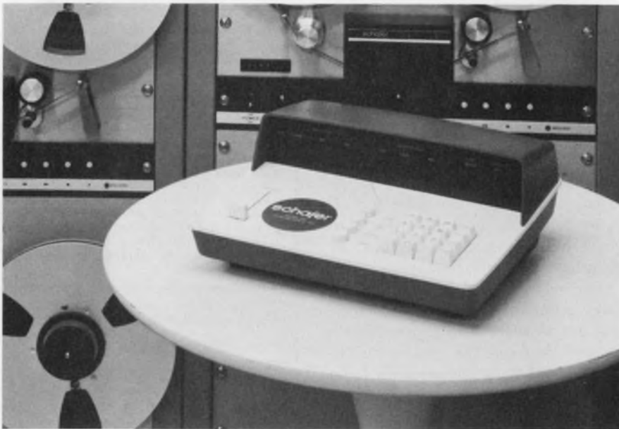
Keyboard memory unit from Schafer Electronics uses an MOS random access memory to store the operating program instead of magnetic tape. The unit holds an entire day's scheduling and can be loaded directly from the keyboard or from a prerecorded cassette.
