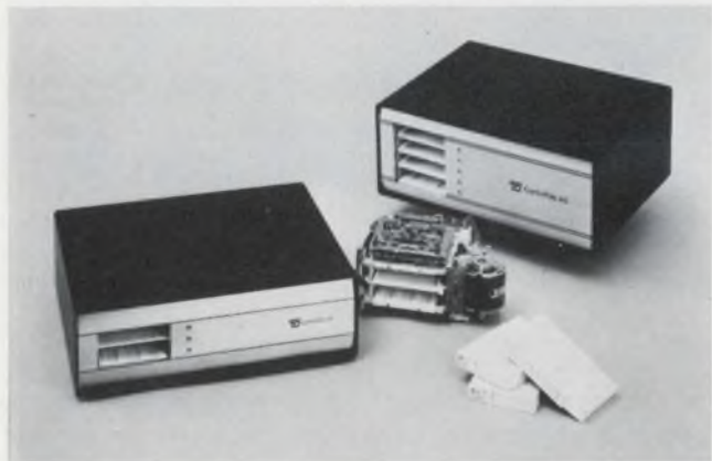
Tri-Data produces several digital cartridge recorders. The drives handle either two or four cartridges at a time. The 1/4-inch tape is contained within the cartridge as an endless loop. Tri-Data's drives all output data in parallel format of either 8, 12 or 16 bits.
