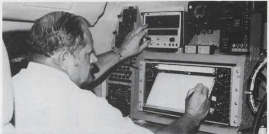
Grumman Ecosystems' manager of systems technology, R. W. Pate, searches for mineral deposits in Peru with Texas Instruments' AN/ASQ-81 magnetometer. In another aircraft the same area is mapped by sidelooking radar.
