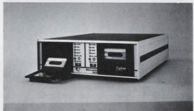
Cipher Data's Mini-cette 2000 is a high performance read-after-write cassette system. It is one of the few cassette recorders that is compatible with the ANSI specifications. It is also one of few recorders that allow recording on both sides of the cassette. One track of data is recorded on each side.
