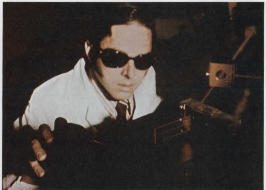
A laser beam is being injected into an experimental optical waveguide by J. E. Goell of Bell Laboratories. The waveguide, made by a masking and etching process similar to that used for ICs, is a deposited glass film.
