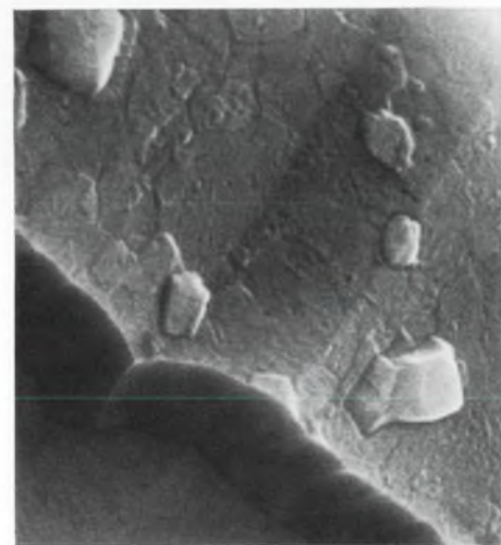
6000 X magnification shows excellent metal coverage over an oxide step. The scanning electron microscope has become a major tool in RCA's diagnostic and high-reliability procedures.
