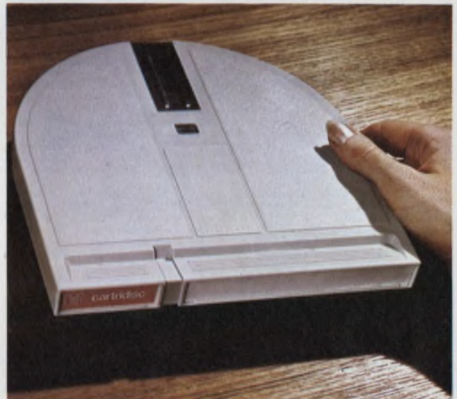
Iomec's Series One, Model 20 drives two 3M cartridge discs. Each contains a flexible Mylar disc that flattens out when spinning. Each disc stores 2 Mb and can be accessed, on the average, in 60 ms. The model 20 contains a master electronics package that can operate an additional six discs in either single or dual-disc drives. Each cartridge disc sells for between $15 and $20, depending on quantity.
