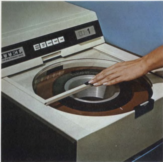
The 733 moving-head disc drive is ITEL's competitor to IBM's 3330. It is an 800-Mb drive with servo-surface head positioning. It uses the IBM 3336 disc pack, with 19 recording surfaces.
