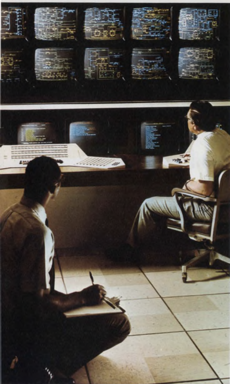
An estimated 10% of all utilities are using or planning to install graphic terminals. Here is a complete dispatch control center, installed at the Philadelphia Electric Co. It was designed by North American Rockwell Information Systems in Anaheim, Calif.
