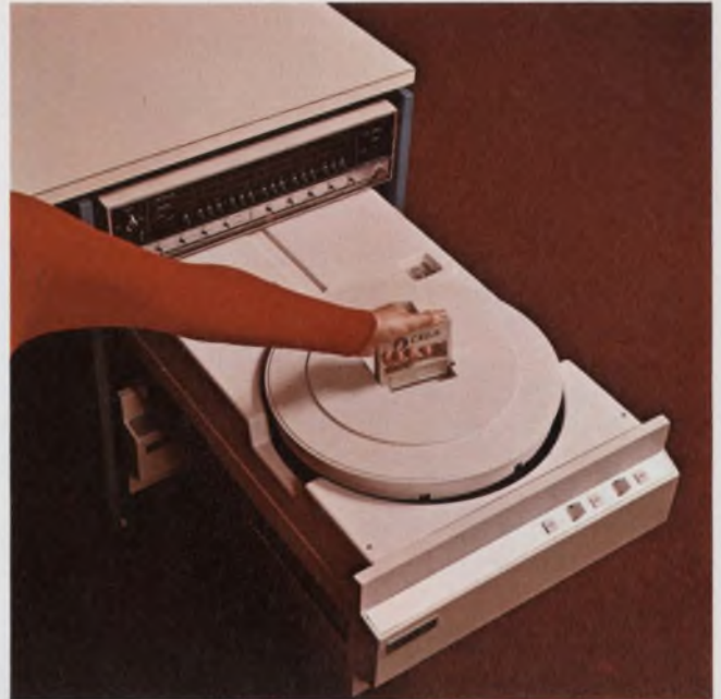
Top-loading cartridges of the IBM 5440 or equivalent are used in the new Caelus 303 moving-head disc system. This memory uses a fixed disc as well as a removable one to achieve 48 Mb of storage capacity.
