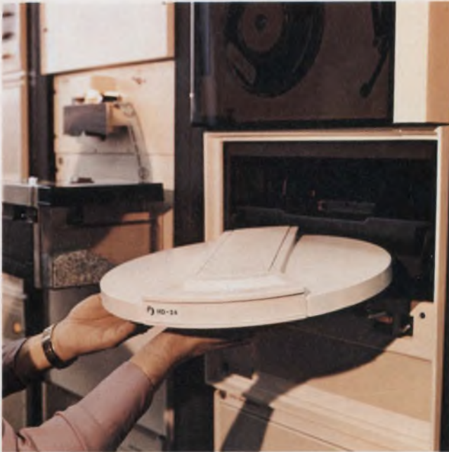
Part of Varian Data Machines' 620/f, Pertec's D5000 moving-head disc drive uses an IBM 2315 front-loading disc cartridge or equivalent. In this case it's a Caelus HD-24 cartridge.
