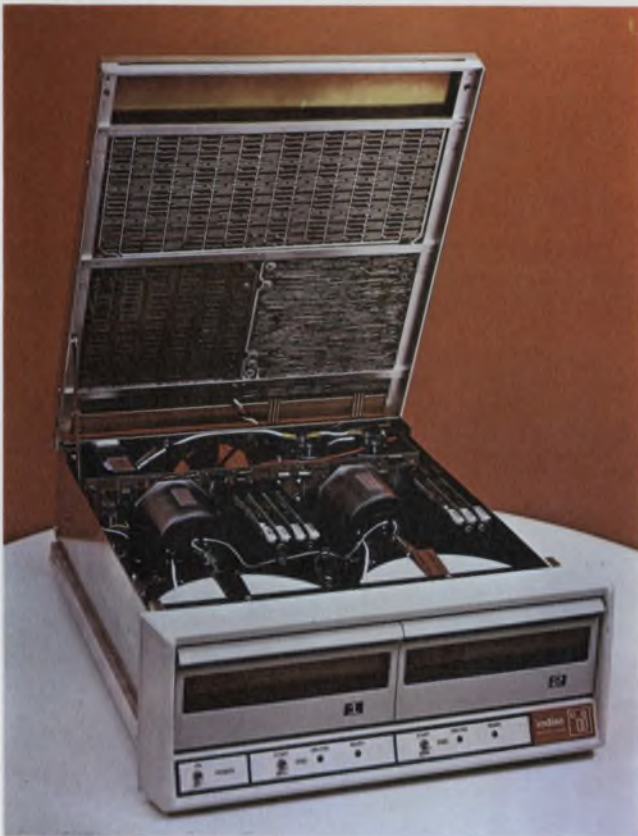
Iomec's Series One, Model 20 drives two 3M cartridge discs. Each contains a flexible Mylar disc that flattens out when spinning. Each disc stores 2 Mb and can be accessed, on the average, in 60 ms. The model 20 contains a master electronics package that can operate an additional six discs in either single or dual-disc drives. Each cartridge disc sells for between $15 and $20, depending on quantity.
