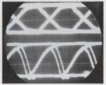
5. Eye patterns reveal the dynamic response of the logic. A random input waveform is at top and the response at bottom. The output lacks the clearly defined "eye" of the input. Clock rate is 50 Mb/s.
