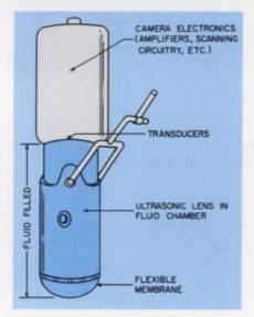
The lower half of this ultrasonic imaging camera is filled with fluid to transmit the high-frequency signals to a patient's body.
