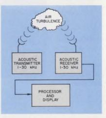
Acoustic radar for detecting aircraft wake turbulence.
