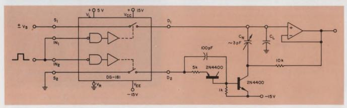
7. This neutralization circuit is almost perfect over a  $\pm 15$ -V signal range. It uses a dual driver and the DG181
