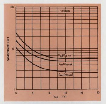
3. Capacitance vs gate-to-source voltage for 2N4091, 4391 and 4856 JFETs.  $C_{rss}$  is the gate-to-source capacitance;  $C_{iss}$  is the sum of gate-to-source and gate-to-drain capacitances.
