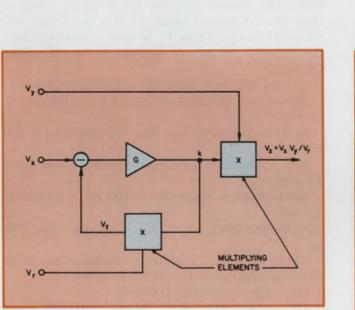
1. Every servo multiplier employs two elements to multiply two signals  $V_x$  and  $V_y$ . The element in the feedback loop normalizes the product with respect to  $V_r$ .
