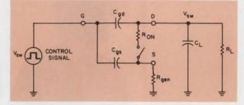
1. Gate-pulse edges form switching transients as they are coupled to the load through FET capacitances.
