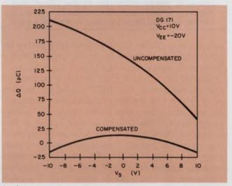
9. Compensation with the circuit in Fig. 10 reduces transferred-charge variation for PMOS FETs like the DG171, with ON resistances of 40 to 100  $\Omega$ . Variation in transferred charge is greater for the uncompensated DG171 than for the uncompensated DG181 (Fig. 8) and full compensation is not as complete.
