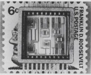
This dual muliplier/divider (5/8 by 5/8 flatpack) is used by General Electric's AICS department on several aerospace programs for precision analog computation.
