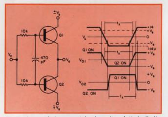
4. Bipolars switch accurately, in spite of their limitations. Output ( $V_{\circ}$ ) waveforms depend on the polarity of the voltage to be switched,  $V_{\rm s}$ .  $V_{\rm 01}$  is the output with  $+V_{\rm s}$  on the collector Q1.  $V_{\rm 02}$  is the output with  $+V_{\rm s}$  on the collector of Q2.
