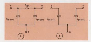
2. The ON (a) and OFF (b) equivalent circuits of a JFET are useful in the noise analysis.
