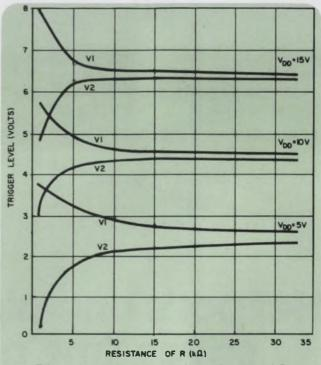
2. Trigger levels plotted against resistance of R for three values of dc supply voltage  $V_{\rm DD}$ . V1 is the ON trigger, V2 is the OFF.
