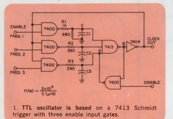
The clock runs until the disable input goes high. If disable goes high when the clock is low (node B high), the positive feedback maintains this state. If disable goes high when the clock is high (node B low), nothing happens until the clock is again low. The system is then latched in the quiescent state. This insures that an integral number of full-width clock pulses is generated, thus eliminating chopped pulses.
