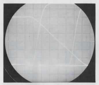
3. The  $t_{\rm PLH}$  of a typical TTL gate increases from 10 ns to 20 as the input fall time increases. The dotted line in this double exposure is the 1.5-V reference level.
