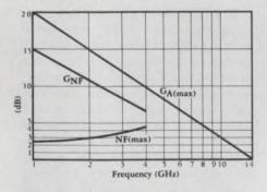
guaranteed noise figure of 4.5 dB at 4 GHz with 6.5 dB gain when biased for optimum NF (10 V, 5 mA). With 3 dB more gain across the band than the HP 21, the HP 22 is useable to 8 GHz in its stripline packages. All for just \$75 each. No other transistor can make that statement.
