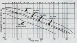
Harris wide band general purpose op amps offer: ■ Close loop bandwidth up to 100 times greater at the same gain or 100 times greater gain capability for the same bandwidth than the common 741 types.
