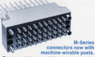
The latest addition to our M-Series connectors gives you real production economy. They have posts for automatic machine wiring . . . four sizes: .022" x .036"; .031" x .062"; .025" square; .045" square.
