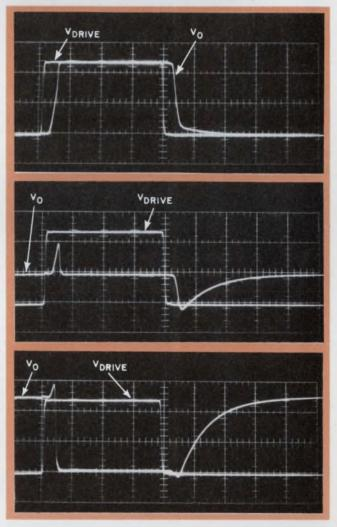
5. Transients in a typical fast JFET switch, the GD187. Here R<sub>L</sub> = 10 k $\Omega$ , C<sub>L</sub> = 30 pF and the scales are 2 V/div and 500 ns/div. From top to bottom, V<sub>A</sub> = +5.0, and -5 V.
