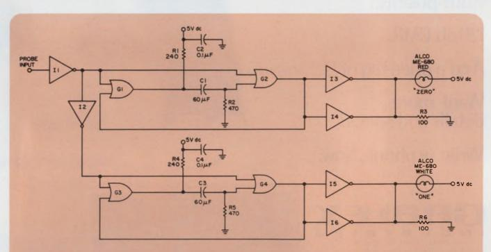
With TTL input pulses, the white bulb winks to indicate the ONE state. Similarly, the red bulb indicates a ZERO. The circuit also indicates logic-level shifts, with the lamps indicating the dominant level.
