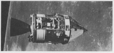
The Lunar Sounder radar will orbit the moon in Apollo 17's service module, similar to the Apollo 15 module shown here. Retrieval of the radar's film will require a walk in space from the command module and back.
