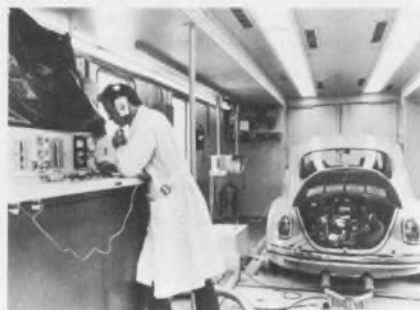
Technician in the trailer unit checks constant-volume-sampling instrument, which collects exhaust gases from the car undergoing test on the dynamometer.
