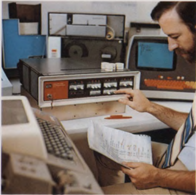
Alpha 16 minicomputer from Computer Automation is a dressed-up version of the Naked Mini 16. The machine is the same in all respects, except that it comes with a control panel and is not meant to be taken apart.
