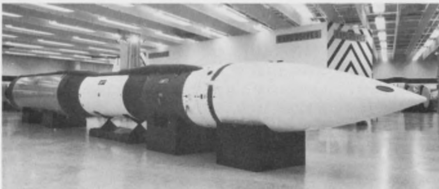
Boeing-built mockup of the Air Force Minuteman III, newest version of the three-stage solid fueled ICBM, shows its bullet shaped shroud, which covers its re-entry system.
