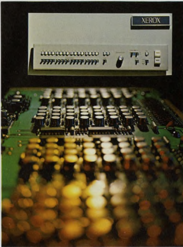
CF 16A minicomputer from Xerox Data Systems is a 16-bit, 1.6- \mu s machine designed for system applications.
