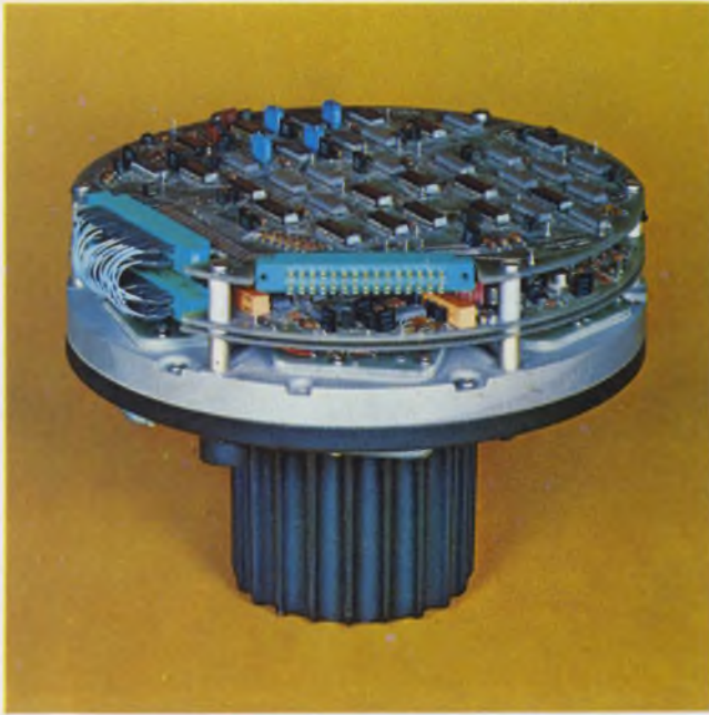
Fixed-head-per-track minidisc memories , such as this Singer Librascope L 107A, with 7 million bits of memory, have become quite popular for use with minis.
