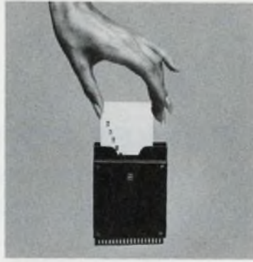
Panasonic's optical static card reader
