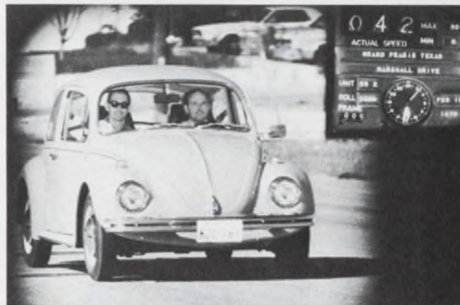
single 35mm movie frame (right). The device, developed by LTV's Missile and Space Div. uses an illumination system operating in the near IR.
