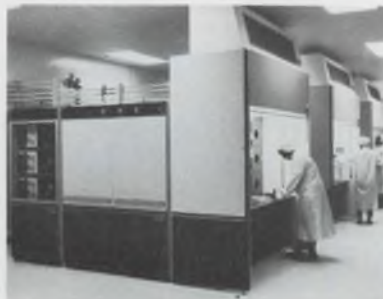
... THE LATEST DIFFUSION EQUIPMENT Six furnace chambers on each of these Brute diffusion systems are regulated within 0.25^{\circ}\text{C} for precise uniformity of wafer diffusion rates.
