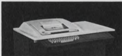
Inktronic® data terminals: A unique electronic, solid state terminal. Prints up to 1200 wpm. Forms characters through electrostatic deflection (no typebox). ASCII compatible.
