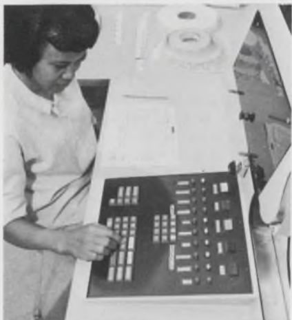
NCR 747 tag printer for new point-of-sale information system automatically produces string-type, pin-on and adhesive price labels.
