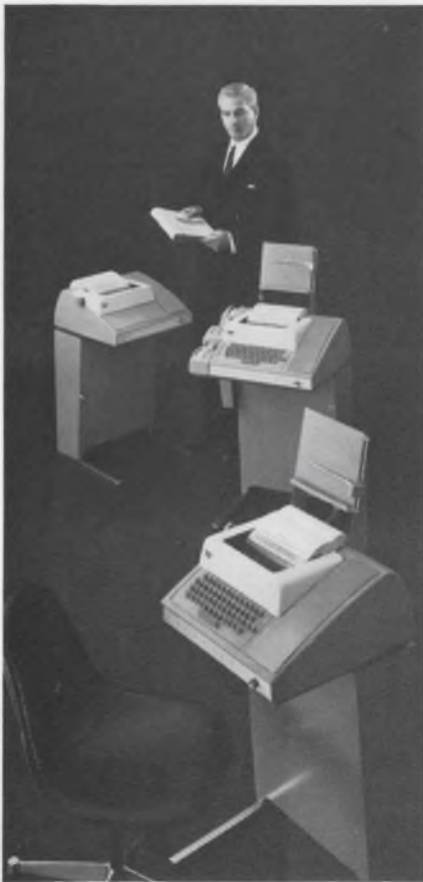
model 33 series: An extremely economical 100 wpm terminal line. Has 4-row keyboard, uses 8-level ASCII code. The most widely used terminal in time-sharing systems today.
