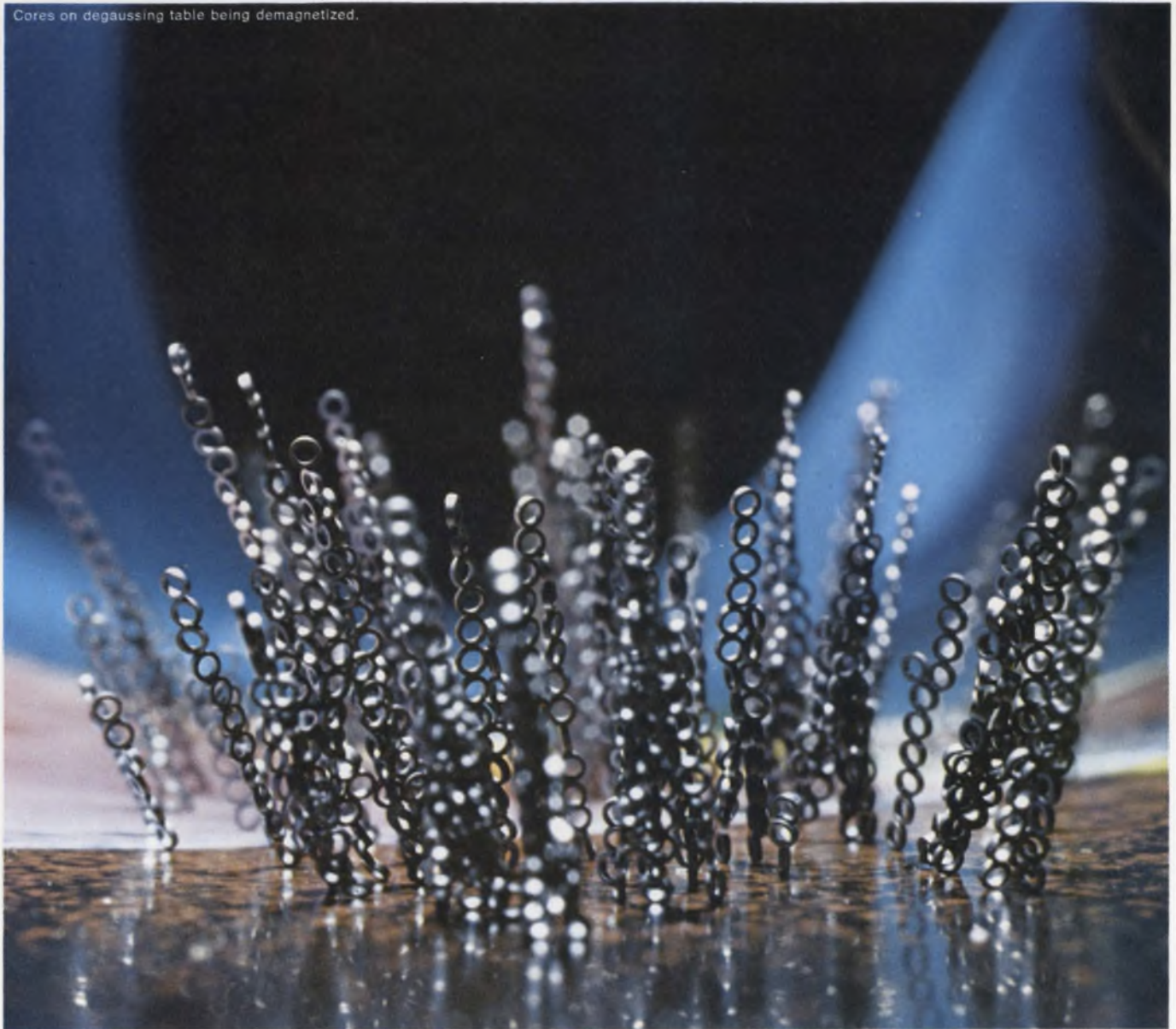
Cores on degaussing table being demagnetized.
