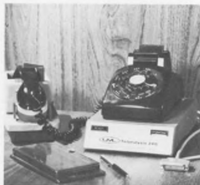
An unattended answering device, the Telanalysis 240, "answers" the telephone in a doctor's office, and an operator at the United Medical Laboratory—a large mail-order laboratory in Portland, Oregon—transmits the results of a lab analysis at any time of day or night to any part of the U.S. It rents for $15 per month.
