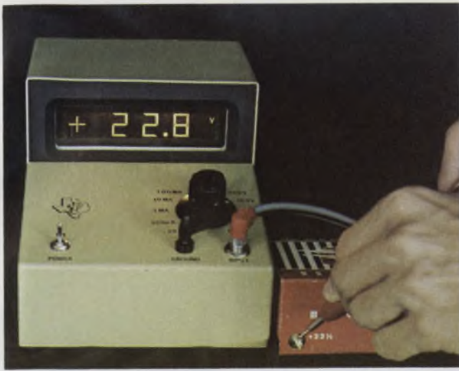
Seven-segment liquid crystal displays from Texas Instruments are incorporated into an experimental digital volt-ammeter. These readouts are back-lighted. Turn-on time is about 2 milliseconds.
